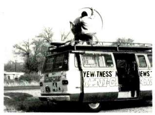
Raising the 2 GHz microwave transmitting dish and aligning it towards the receive site on Sandia Crest.
