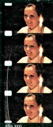
A 1000 100-watt bulb 6 ft. over model's head. 5 motcandles, f/1.4 ed 3 stops
