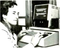
Ham operator Mike Slefian, on duty in the Emergency Control Center, enters a warning report into the character generator. Message appears simultaneously on read-out screens in WBEN news and master control.
