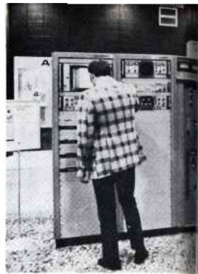
Harris' BT-25L1 VHF transmitter.
