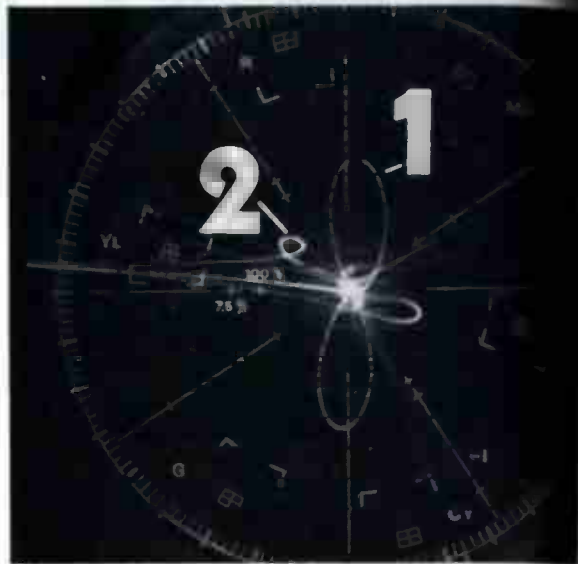
Fig. 1 Expanded center of color bar showing "Bow Tie" leading edge of grey Bar (No. 1) and modified "Bow Tie" sync (No. 2). Note absence of jitter both with respect to other and also over the two-field period of the exposure.
