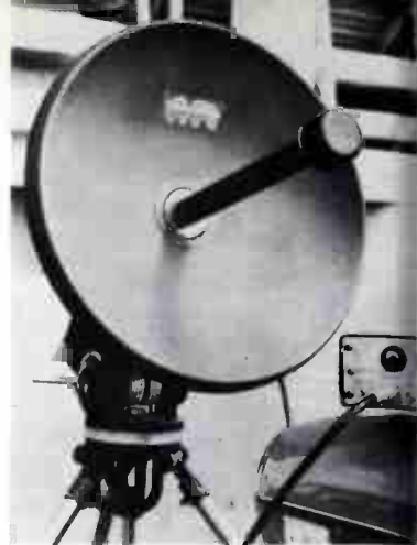
Terra Com's compact portable ENG transmitter.
