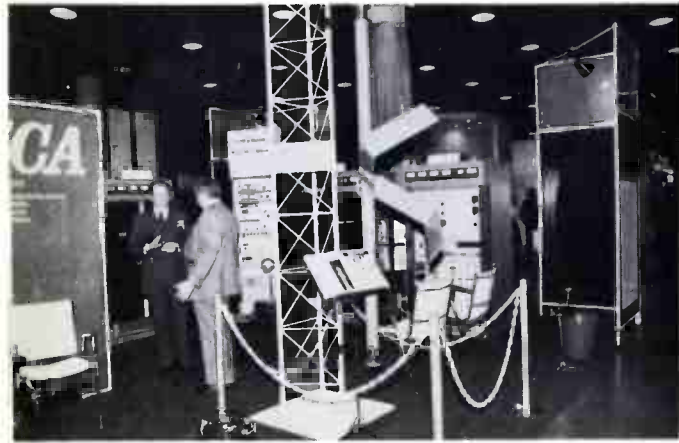
CCA had hi-power FM antenna with "strap" elements.
