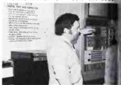
CVS 20 TBC has 9 bit sampler at 4x subcarrier.
