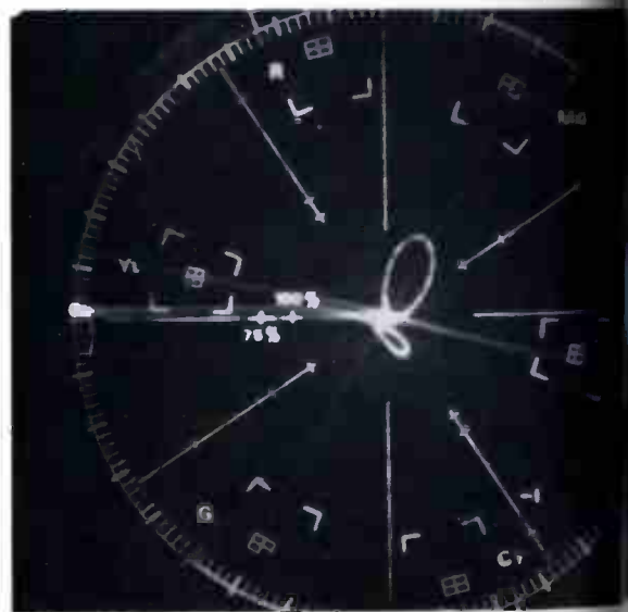
Fig. 2 Expanded center of color bar. One (1) line of 52.5 half of "Bow Tie" from Grey Bar (luminance) and half of B from sync. Photo time is one second. Therefore, this is the line integrated 15 times. Note stability is excellent of all components (burst, sync, luminance).
