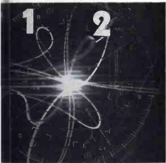
Double exposure of a color bar signal before and after through a proc amp. Note: No. 1 is sync incoming No. 2 is sync outgoing—3 degrees or approximately 2.4 Subsequent recording and playback results in jitter added to the picture with jitter free sync added stable for subsequent generations of tape.
