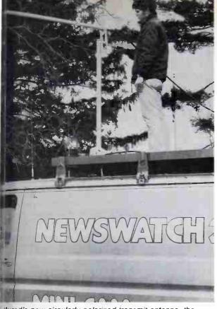
Nurad's new circularly polarized transmit antenna, the Boldenrod.
