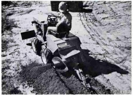
18-HP Model J20 — 4 wheel drive, with three speed forward plus reverse transmission Ditch Witch . . . equipment from 7 - to 195-HP.
