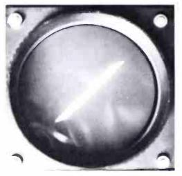
Fig. 5 Trace shown is composite of 150 Hz, 1 KHz and 8 KHz; switching oscillators on and off will reveal that the component at less than 45° Is from an 8 KHz tone that is much lower in one channel.
