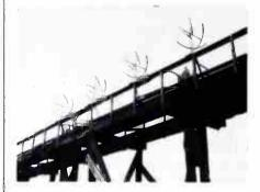
Rocamora, RCA antenna engineering manager, said that the new design is cheaper than a panel-type unit, has lower wind loading. The antenna will have eight bays, each with radiators more than twice as large as those in previous single-station antennas of the type. The photo shows several of the antenna bays under test at RCA's Gibbsboro antenna facility.
