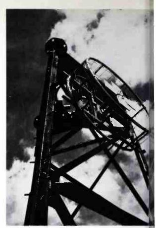
Harris CP antenna has crossed dipoles backed by a cylindrical cavity formed of open wire to reduce wind loading. Rotating field from dipoles excites cavity, which it in projection of CP signal at high efficiency.
