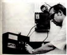
FSM-2 has accuracy of ± 1.5 dB and readings from 10 microvolts to 3 volts. Front panel switches choose average or peak, VHF or UHF, and 110 volt AC or battery operation. DC output connector will feed a graphic recorder and modulation test jack.
