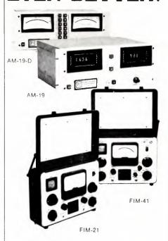
FIM-21 Field Strength Meter, 535 KHz to 1605 KHz Lightweight, easy-to-use, the '21' is the new solid state replacement for the time-proven Nems-Clarke FIM-120 (RCA WX-2). Using six standard D cells, the unit features a ceramic IF filter, ganged osc/receiver tuning, front panel speaker and illuminated meter and dial. Field strength values between 10 microvolts/Meter and 10 volts/Meter. An external RF input jack is provided for tunable voltmeter applications.
