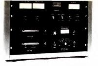
Heart of any FM transmitter is the exciter. Pictured above is one of the latest to be designed, the FME 10 (lower chassis) coupled with a 60W amplifier to make up an all solid-state FM transmitter. Unit is from Wilkinson.
