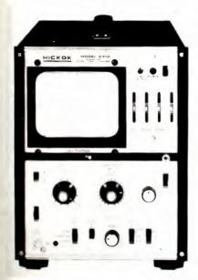
stable triggering to 15 MHz. Model 5310 has vertical sensitivity from 10 mV/cm to 50 volts/cm in 12 calibrated ranges, with accuracy ± 3%.
