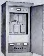
Emcee's solid state 2500 MHz transmitter.
