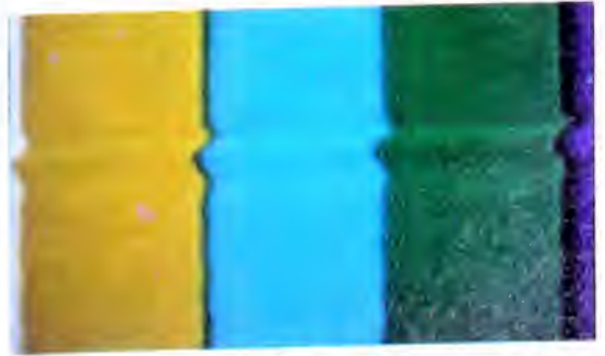
Stability of the SECAM/60 hue with severe timebase error can be seen in this color bar picture, made with deliberate disturbance of video head drum
