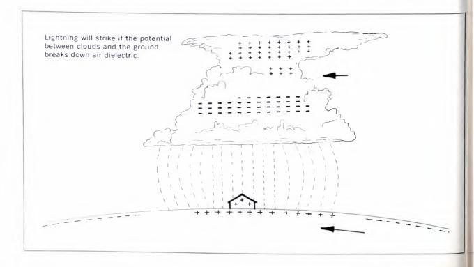
ubstantially reduced. This is just what the LEA ystem sets out to do, with an array of very many harp metal points, connected to the ground and pointing upward. The ability of a sharp point in a trong voltage gradient in air to start a current across he gradient has been known since Ben Franklin lew his kite. The LEA dissipation array "leaks" the charge across the air gap.
