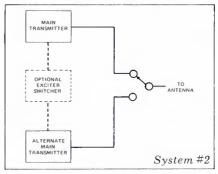
unit. Also, the availability of two identical transmitters simplifies servicing by providing a cross-reference for testing and evaluation of performance.
