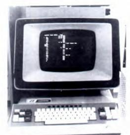
Close up of the Vital Vimax-27 console. The 27 events that this system handles are more than adequate for WLWD's chief engineer, Harold Thompson. take. With this system, the needed entry is a bare minimum. In the example just cited, Net and Time were all that were needed for the full event.
