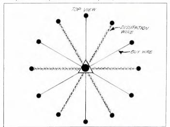
Diagram shows six dissipation wire radials strung from antenna (held up by guy wires). Antenna height is 225 feet. Dissipation wires are insulated from the tower and form angle of 35 degrees with respect to the ground.
