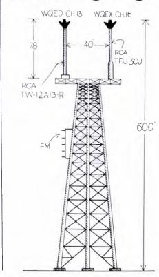
A self-supporting tower and antenna system with a unique "T-bar" structure is now under construction for Pittsburgh's two educational TV stations—WQED and WQEX.
