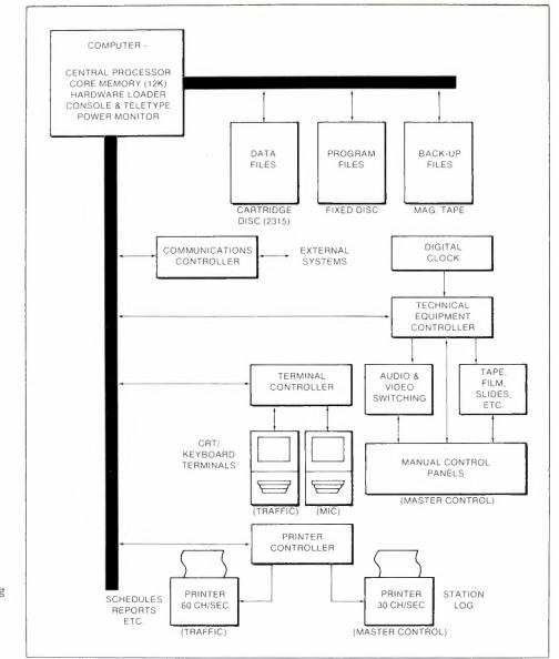
Simplified diagram by Central Dynamics of key elements of free-standing computer system.
