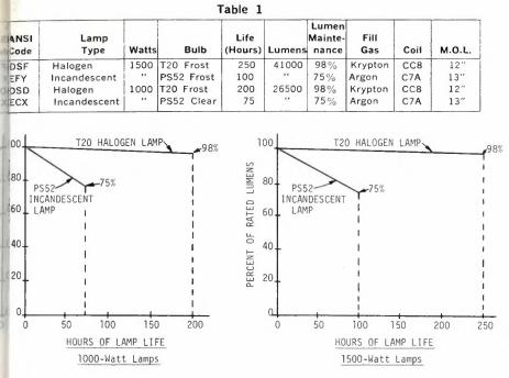
Fig. 1. Halogen lamps have longer life than incandescent counterparts.
