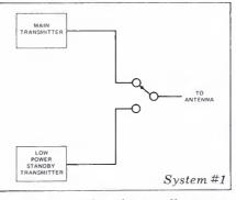
a-week inspection, the standby transmitter must be capable of delivering at least 20 percent of the station's licensed power.
