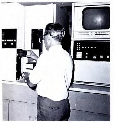
Semi-automatic broadcasting of break material: The Ampex ACR-25 cassette broadcast videotape recorder/player holds up to 24 cassettes that can be player manually, semi-automatically, or automatically. The unit pictured is the first of its kind to be delivered. It's at KTEW, Tulsa, Oklahoma.
