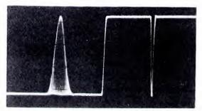
Input and output waveform characteristics for 2T luminance and 10T chrominance pulses.
