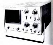
by input control switch; chopped or alternate presentation is automatic, depending on time base. Bandwidth is 10 MHz, sensitivity 50 mV/cm. Tentimes sensitivity magnification, and five-times sweep magnification are available. 500 volts peak input can be accepted indefinitely. PHILIPS. 290
