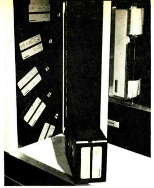
View of transport with carrousel door open and five cassettes installed.
