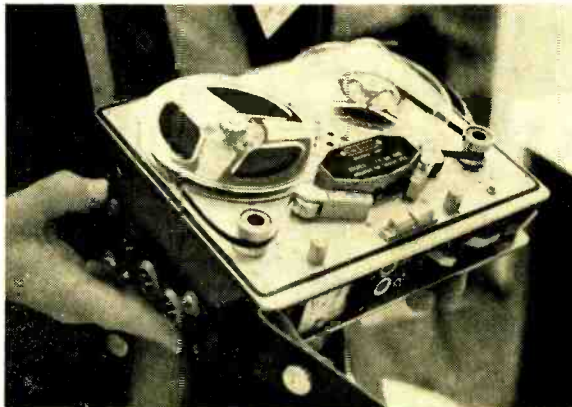
Available in mono or stereo versions, the Stellavox SP-7 has four speeds: 15, 7 1/2, 3 3/4, and 1 7/8 in./s. Reel size is 5 in. with cover closed, up to 10 1/2 in. with cover off and using adaptor. Close speed control, balanced mike input, wide frequency response are other features. Cost of mono non-sync model is approximately $1500.
