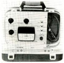
band fm electronics with center frequency carriers up to 432 kHz. Independent three-point calibration of modulators and demodulators can be performed as well as overall fm channel calibration. Zero center meter provides plus and minus three percent full-scale maximum error readings. \$550. Micom, Inc.
