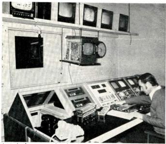
A stack of programmed pinboards sits ready for the switcher. Boards will control three VTRs, film projector, slides and audio gear.
