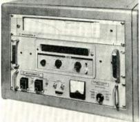
set frequencies minimizing cochannel interference. System consists of high precision oscillator, strip chart recording receiver which continuously monitors U.S. standard station WWVB in Boulder, Colorado, and an electronic counter showing station's output at any given time. Transmitter stability is as much as 10,000 times FCC requirement of ±1000Hz. Drift rate on channel two station is less than 0.2Hz per week at carrier frequency. Motorola Communications and Electronics,
