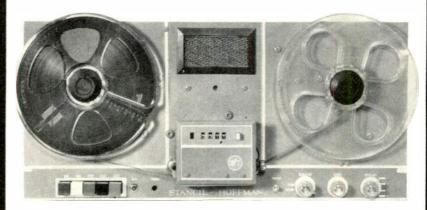
Here's a full 24 hour, 4 track logger that's so compact and versatile you can take it anywhere to handle any assignment with 100% dependability or rack mount it in the studio. A remarkable new series of silicon transistor plug-in amplifiers makes the R-70 the most versatile ever—AGC, recall, full remote or automatic control, stereo, fail-safe, synchronous time injection, etc. 4 channels round the clock, complete on just one 7" reel of 1/4" tape.
