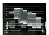
Type 528 Waveform Monitor Display of split-field color bars per EIA Spec. RS189. Signal source — Type 140 NTSC Test Signal Generator.
