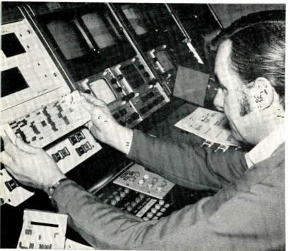
Changing pinboards in WXTV's master control takes only a few seconds, and can be done while an automated event is in progress.
