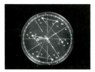
Type 520 Vector Display of VITS color bars conforms to EIA Spec. RS189. Signal Source — Type 140 NTSC Test Signal Generator.
