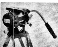
head is made principally of magnesium alloy, tilts 45° up and down, and pans 360°. Both pan and tilt drags are indefinitely adjustable. A torque rod, capable of providing up to 200 in. lb is provided for counterbalancing camera tilt. Head has snap-action camera platform.
