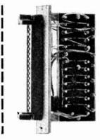
AA-601 Plug-in Audio Distribution Amplifier Module (with cover removed) — self contained, solid state design. Each module provides up to 6 outputs (60 in a 51/4" frame) at  $\pm 24$  dbm, 600 ohms balanced.
