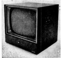
lage, Ill., provide horizontal line resolution of 800 lines at center screen. Prices range from \$499.95 for the 17-in. monitor to \$549.95 for the 23-in. unit. A 27-in. vacuum tube model also is available for \$499.95. All moni-
