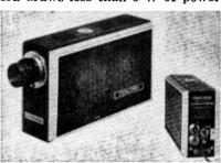
and has a vidicon tube whose is 3000 hr. Camera is equipped with an F 1.8 25mm lens, and may be optionally equipped with a low-cost zoom lens. Resolution is 550 lines. Camera has output impedance of 75 ohms; minimum light intensity is 40 lux. Camera weight is 6 lb. MTC-15 is priced under \$400.
