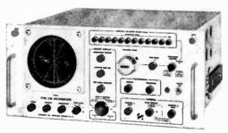
Measuring amplitude changes and phase shifts can be done accurately, conveniently, and independently with the Vectorscope. The Vectorscope presents relative phase and amplitude displays (of chrominance Information in the N.T.S.C. color signal). Dual-trace capability permits simultaneous display of two color signals for precise matching of phase and amplitude. In addition to the vector display, the Vectorscope can present the chroma signal demodulated along any phase-angle with respect to time.
