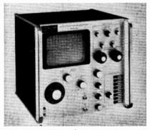
Hz, manual, and external sweep rate. Unit has crystal controlled marker generators for frequency identification; provision is made for eight single-frequency plugin markers.
