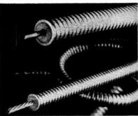
50-percent more flexible than conventional noncorrugated coaxial cables. Coro-Flex with OD of 0.500 in takes bends as small as 2½ in. dia without electrical or mechanical discontinuities. Cable terminates with type F connectors and has impedance of 75 ohms. The smaller 0.325-in. OD cable is electrically similar to RG87A/U and has 50 ohms nominal impedance. Smaller cable terminates with type N connectors.
