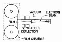
coating on a CRT screen. Designated the EBR 100, the unit weighs 1000 lb and has a 16mm film capacity of 1200 ft. Results indicate that the EBR 100 is able to process film six times faster than conventional kinescoping methods, and the resulting pictures have higher resolution, less graininess and noise, and brighter images. The EBR 100 system is priced in the \$60,000 range.
