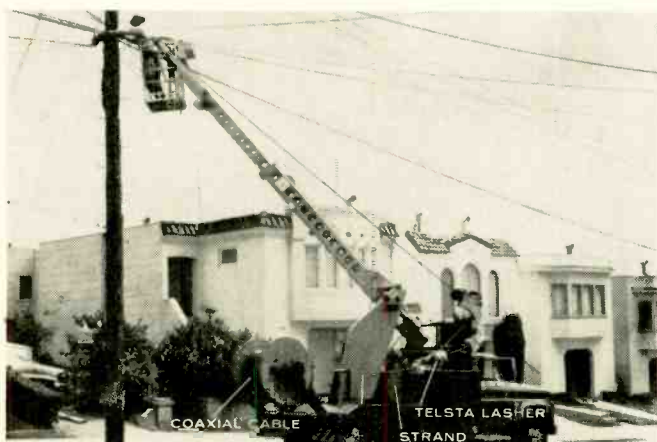
Telsta Corp. manufactures this combination electric lift and Tel-Lasher cable and strand stringing outfit.
