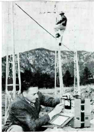
CATV engineers making on-site signal measurements and reception tests.
