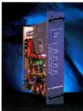
▲ BASIC 1-kW POWER AMPLIFIER MODULE.
