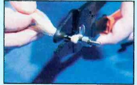
Fiber-optic connector being attached to a fiber cable using Kevlar as a strain relief beneath the crimp sleeve.
