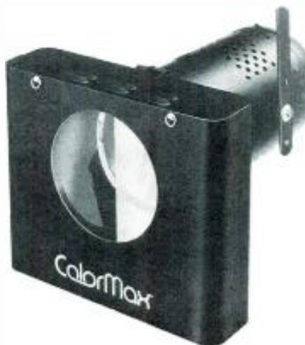
ColorMax is a self-contained unit that slides into the gel frame holder of the lighting fixture. It plugs into a 120Vac non-dim circuit for motor and fan power. The control signal is programmed from an external controller, and up to 100 units may be slaved to a single control channel. Maximum color change time is 2.5 seconds, using all 12 color squares.
