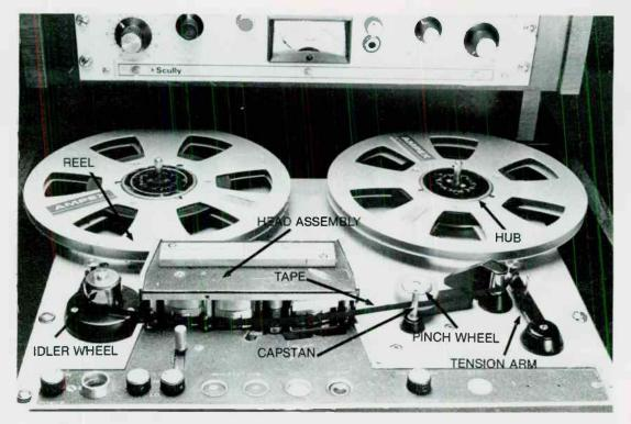
Figure 13.2. Tape Path. (Photo by Pheobe Chase Ferguson.)
