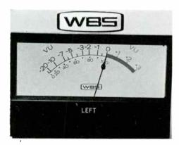
Figure 14.3. 0 VU Meter Reading. A "0 VU" reading on the standard VU (volume unit) meter. Note that the scale above the line is calibrated in dB (decibels) relative to "0" or "reference level," and the scale below the line is calibrated in percentage of modulation for broadcast transmitters. "0 VU" equals 100% modulation. (Photo by Skip Pizzl.)
