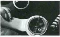
The alligator clip is attached in this fashion to provide the firmest connection. Its teeth grip thightly across the edges of the "tongue," rather than gripping the flat, smooth surface, from which the clip could slide off.
