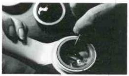
Attaching the first atligator clip to one of the receiver's "tongues."
