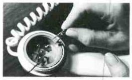
The second clip is attached in a similar manner. It doesn't matter which clip goes to which tongue, as long as the clips don't touch each other.
