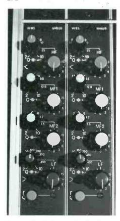
Figure E.1. A Parametric Equalizer (Ward-Beck Systems). This model is built into a mixing console.
