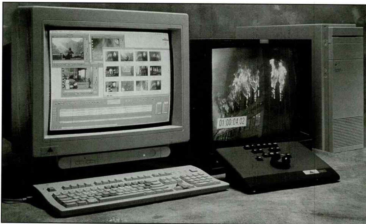
A companion monitor displays time code for each frame of video from a scene in the monitor at left.
