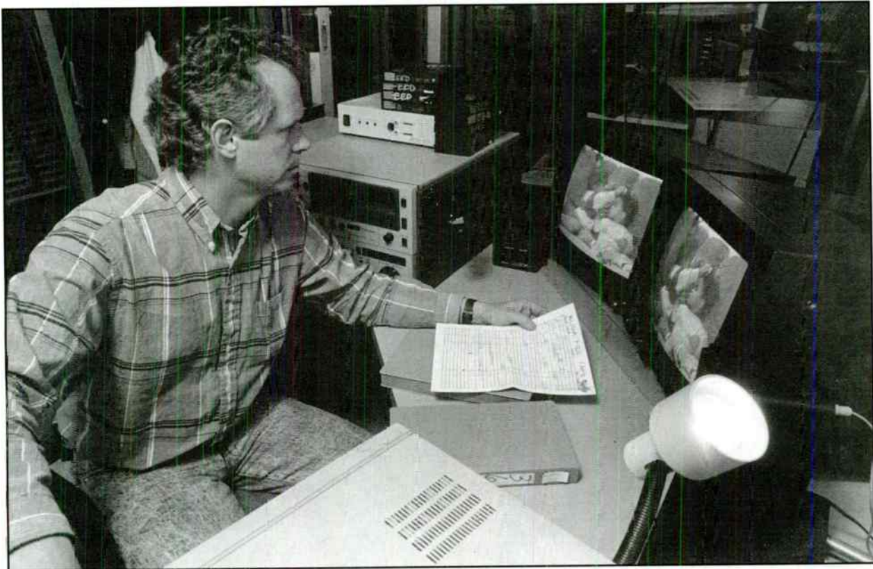
The videotape cassette editing system allows electronic transfer of material from the playback unit onto a master cassette in the videotape recorder.
