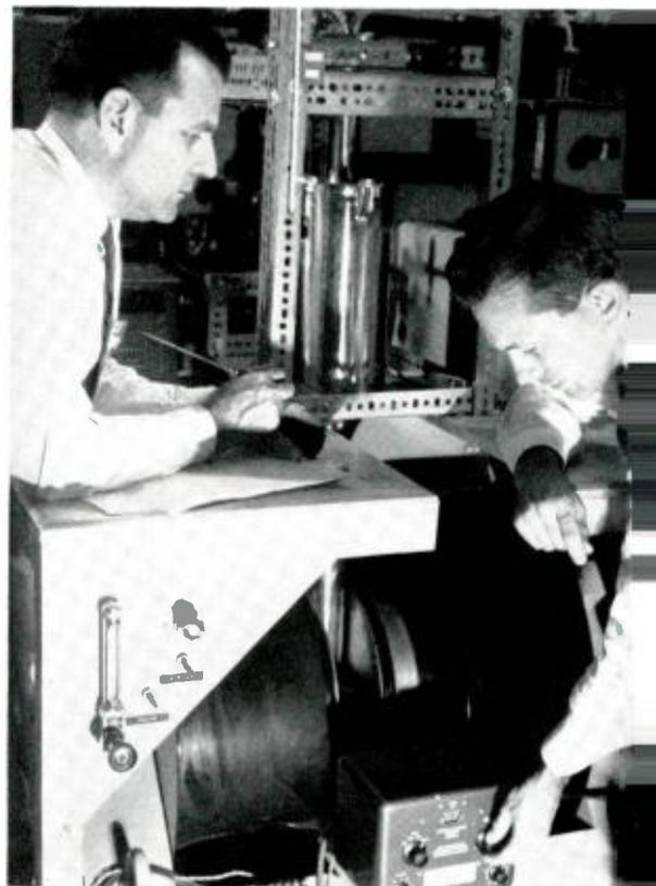
*E. G. Spencer, left, and R. C. LeCraw adjust apparatus with which they measured what appears to be the inherent resonant linewidth of perfect yttrium iron garnet.*
