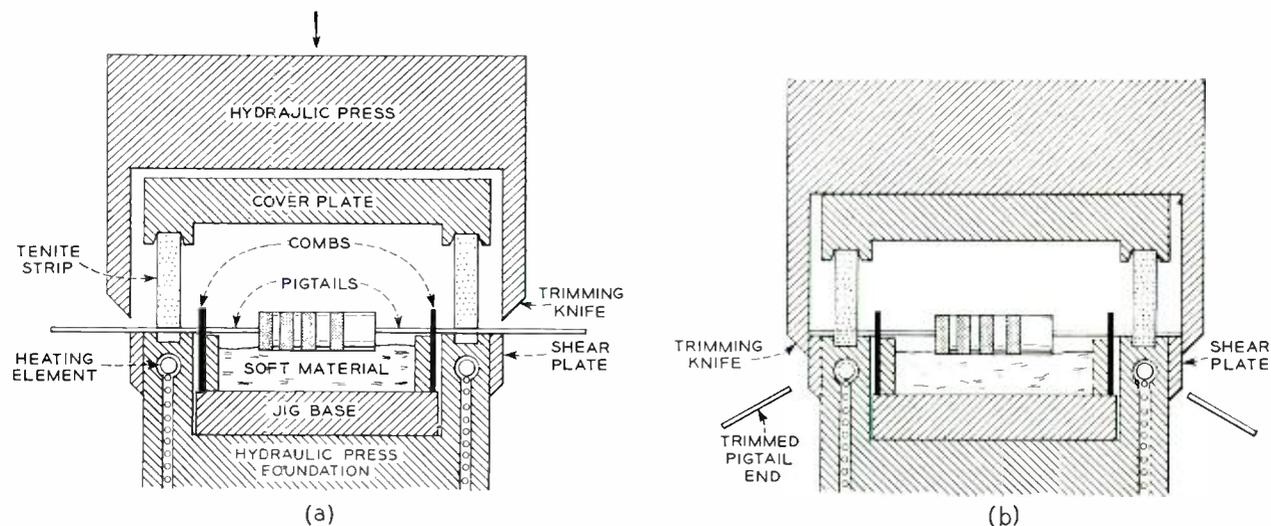
Fig. 4—At the left, a jig with parts and plastic strips is in the machine just before it operates; at the right, the press has forced the heated strips down over the wires and trimmed the wires to length.
