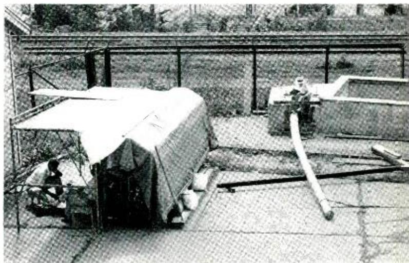
round timbers when tested below fiber saturation. Except for a few of the initial poles tested (which were covered with wet tarpaulins) all poles both treated and untreated will be kept fully submerged in a special soaking tank. They are removed a few at a time and kept wet until just prior to test.
