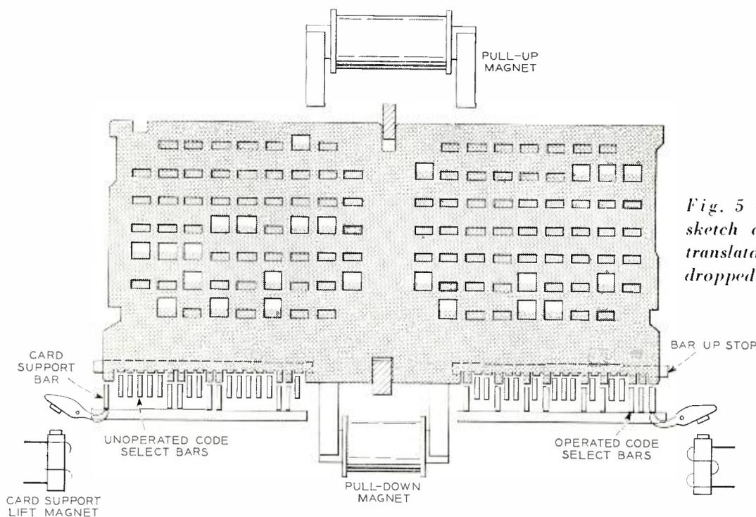
*Fig. 5 — Simplified sketch of end view of translator, one card in dropped position.*
