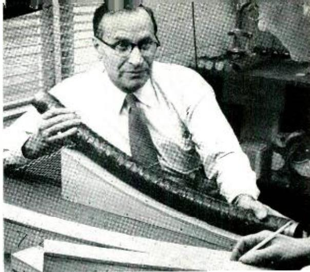
*Scientists examine wood forms used in testing signal transmission around curves through the new “helical” waveguide.*
