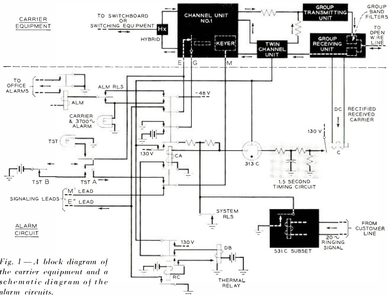
Fig. 1—A block diagram of the carrier equipment and a schematic diagram of the alarm circuits.
