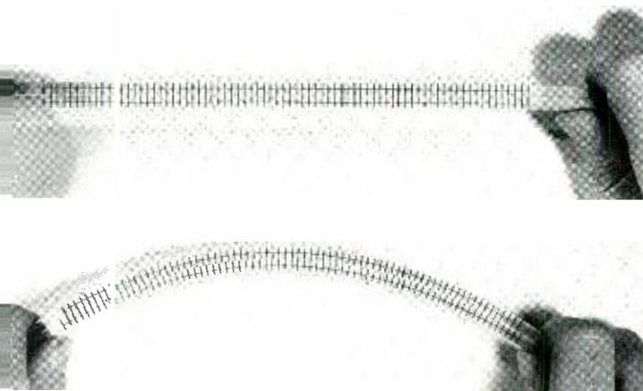
Fig. 5—Flexible bars with ruled lines can be bent to illustrate production of dislocations by bending.
