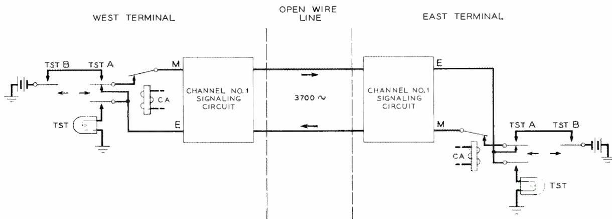
Fig. 2 — Loop testing is made possible by connecting the E and M signaling leads at each terminal.
