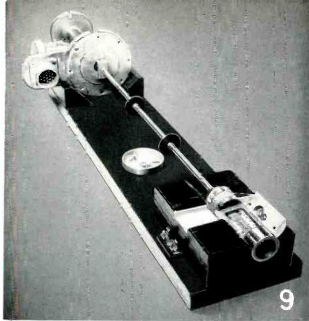
After the bridge is completed, it is mounted in a sample holder, Figure 9. The bridge with the gold contact wires in place, can be seen in the cavity near the end of the holder at the lower right-hand corner of the photograph. The bridge and holder are then placed in low-temperature apparatus for Hall effect and conductivity measurements.
