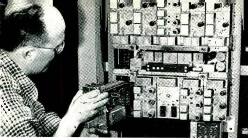
Fig. 4—C. W. Irby removes a twin-channel unit to give better access to the alarm circuit just above.
