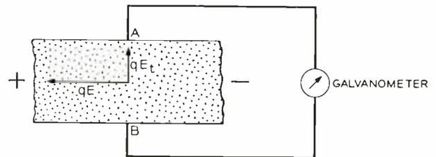
Fig. 1 — Schematic representation to show the Hall effect. Distribution of mobile charges in a ribbon placed in a magnetic field is distorted by the field.
