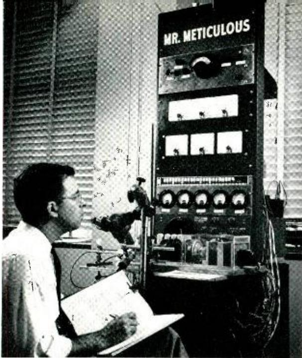
*The new Laboratories' machine for assembling experimental transistors in operation at Murray Hill under observation from R. P. Riesz.*
