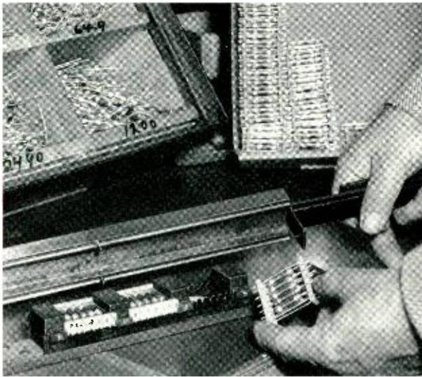
*Fig. 5—Several small assemblies can be made at one time in a jig like this.*
