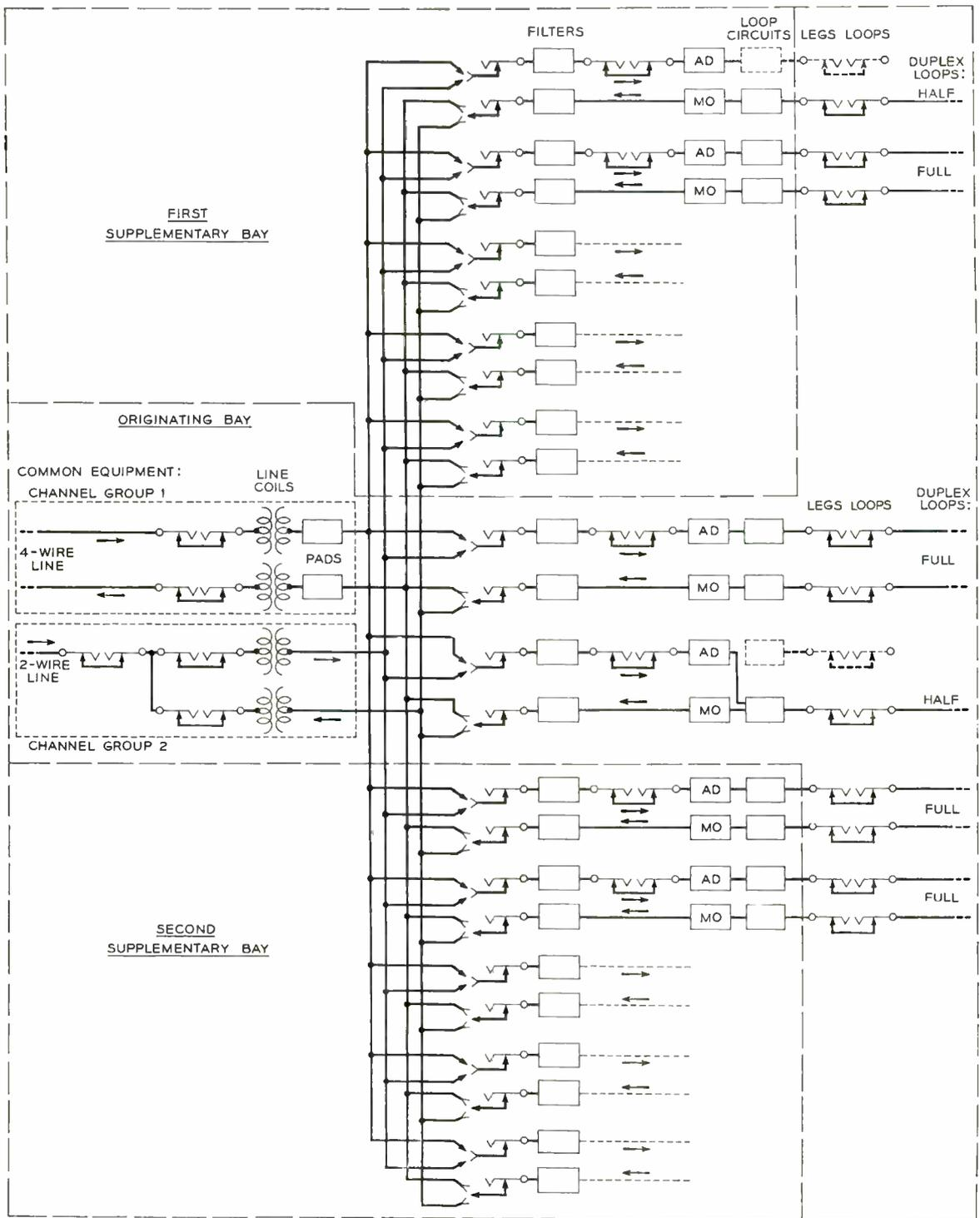
AD = AMPLIFIER DETECTOR, MO = MODULATOR OSCILLATOR
