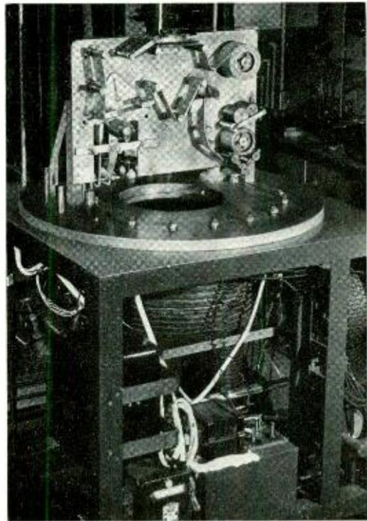
*Fig. 5—Vacuum vapor-plating machine with bell jar and side panel removed. The plating occurs in the upper section normally covered with the evacuated bell jar. Below are located oil diffusion pumps, transformers, speed control and the water-cooling coils*
