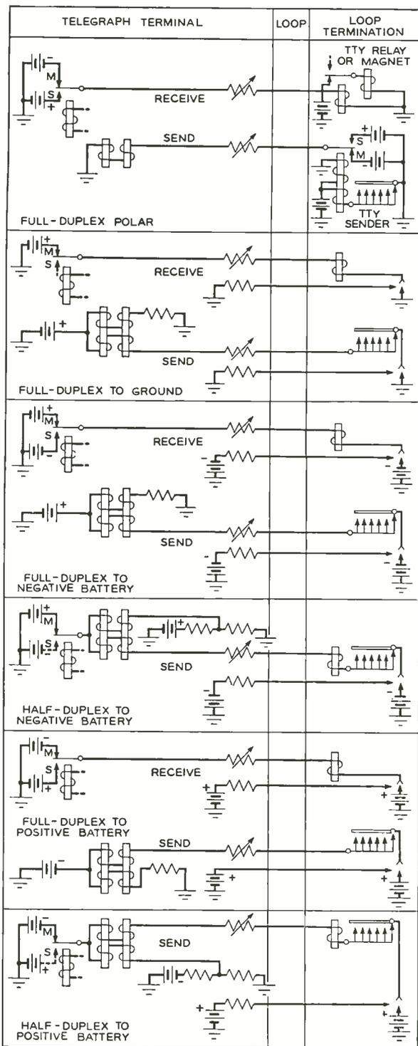
Fig. 4—The six possible loop connections that are possible with the 40AC1
