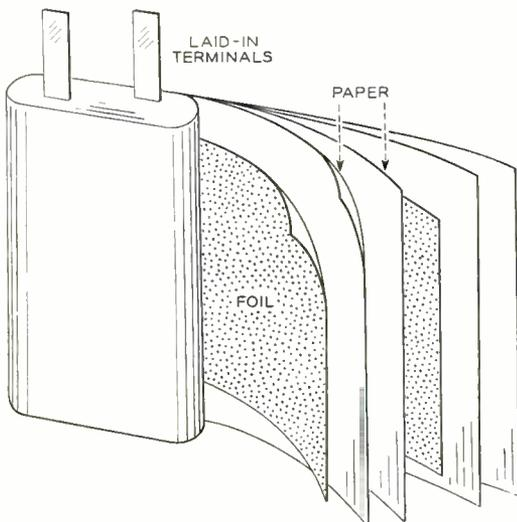
Fig. 1—A foil type capacitor above and a metallized paper capacitor of the same capacitance below. Method of constructing foil type capacitors is shown at the left
