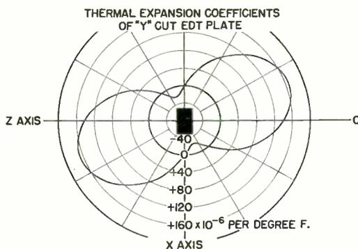
Fig. 5—Thermal coefficients of linear expansion in directions parallel to the major face of a Y-cut EDT crystal plate. The negative Y-axis extends toward the reader
