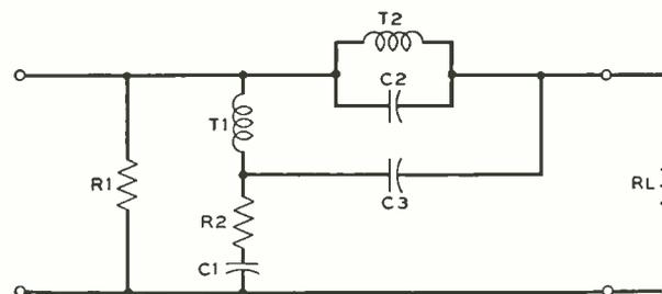
Fig. 3—Circuit of the 103A frequency generator
