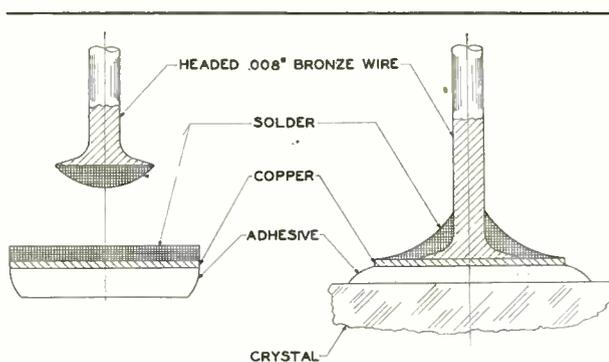
Fig. 4—Left, below, combination adhesive disk before cementing to EDT plate. Left, above, headed wire that will be soldered to the disk's solder layer. Right, combination adhesive disk after cementing to EDT plate and after headed wire has been soldered to the solder layer. Note overlap of adhesive that furnishes proper surface for electrical continuity between mounting wire and gold electrode
