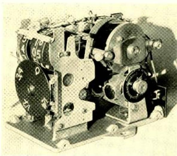
Fig. 4—View of time unit showing cyclometer, at the left, and the adjusting knob and gears for rotating the motor winding, at the right
