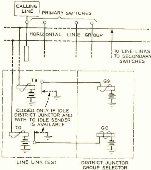
Fig. 4—Idle link identification is made by ten groups of ten pairs of relays
