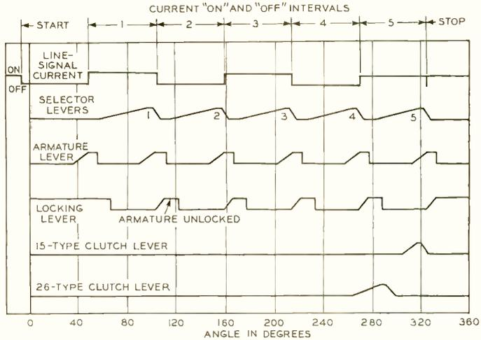
Fig. 3—Timing of the cams of the selector-cam assembly. The relationship between the line signal and the operation of the several cams can be varied by repositioning the range-finder arm of the mechanism
