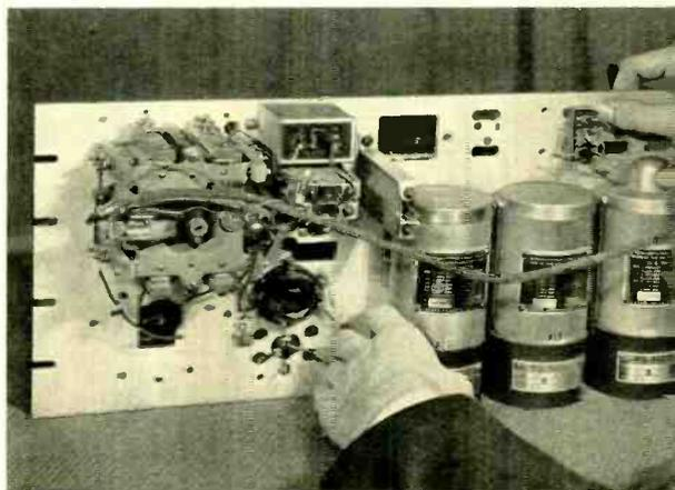
These two models, representing different stages in engineering the 2B Regulator, were built in the Shop. "Breadboard" models were built, but have not survived. As soon as such a model has served its purpose, it generally is disassembled and the apparatus used in a new circuit.
