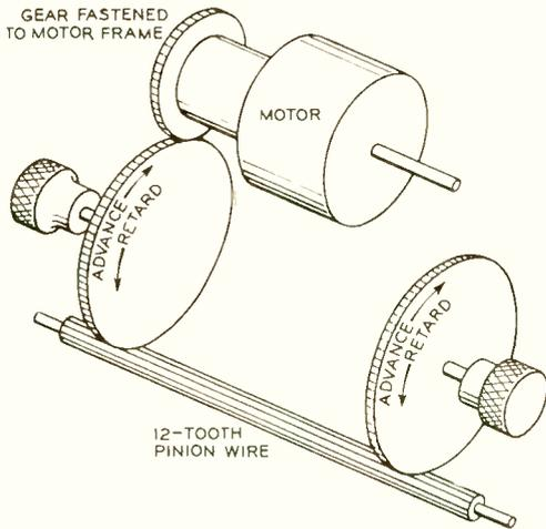
Fig. 5—Gear arrangement for the adjusting drive
