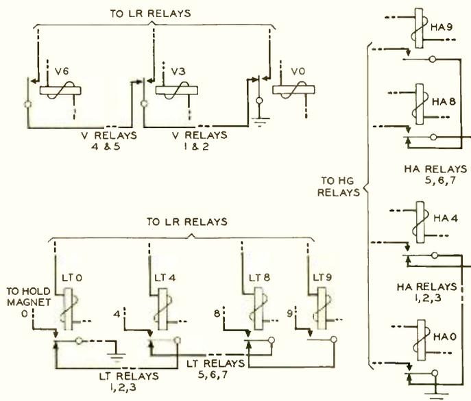
Fig. 5—Typical chaining circuits of the line-link controller
