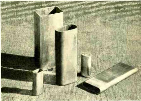
*Fig. 2—Collapsible tubes extruded in the Laboratories Shop. The smallest tube on the right is made of aluminum and the other four are lead*
