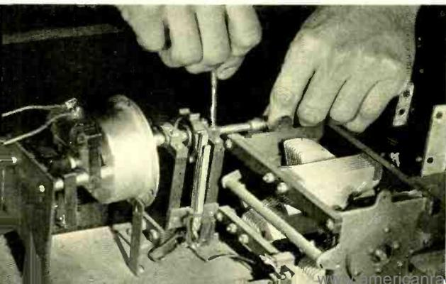
The 2B Regulator, shown at the right, occupies but nine inches of space on a standard relay rack. An entire C5 carrier terminal, including the regulator, is mounted on one bay, as shown below.
