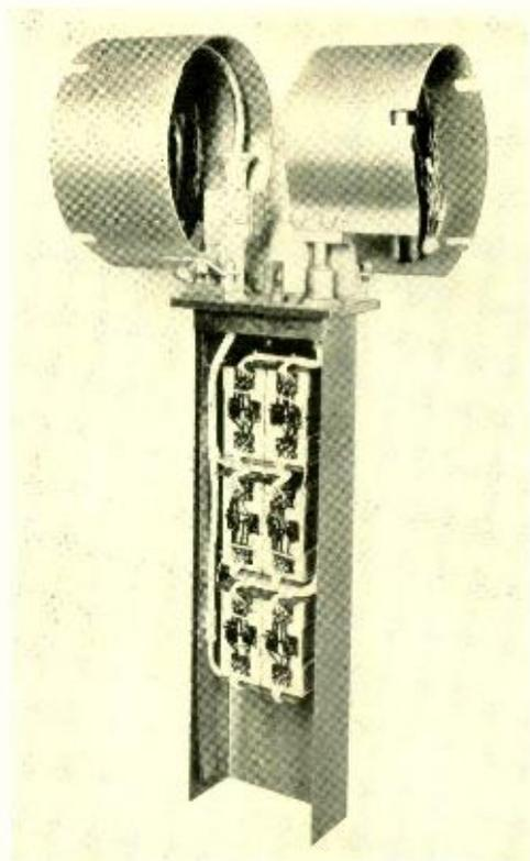
Fig. 4—Partially assembled loading coil case potting six 81A filters
