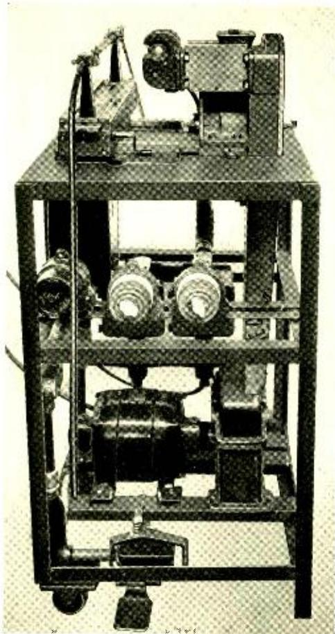
*Fig. 2—The machine for completing paragutta joints applies the plastic material at the rate of about an inch per minute*
