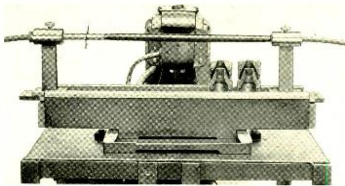
Fig. 3—The two parts of the extrusion die which apply paragutta to a cable joint can be seen resting on top of the machine
