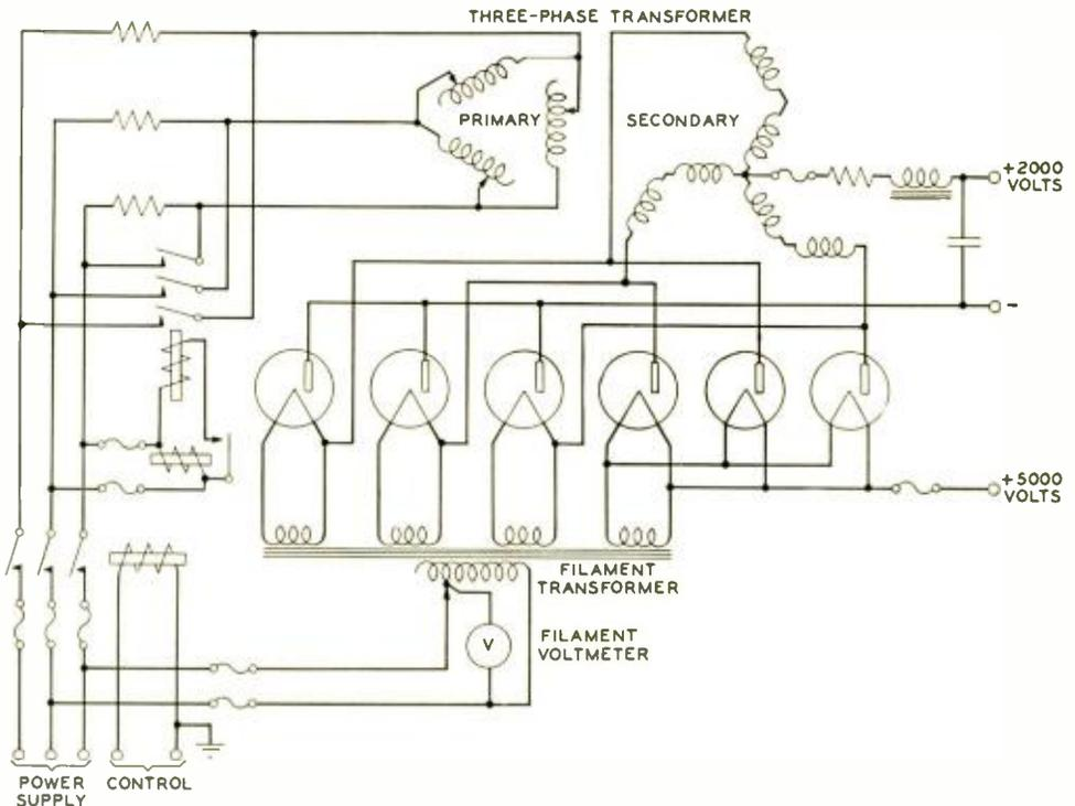
Fig. 1—Simplified schematic of mercury rectifier for the No. 6 type broadcast transmitter
