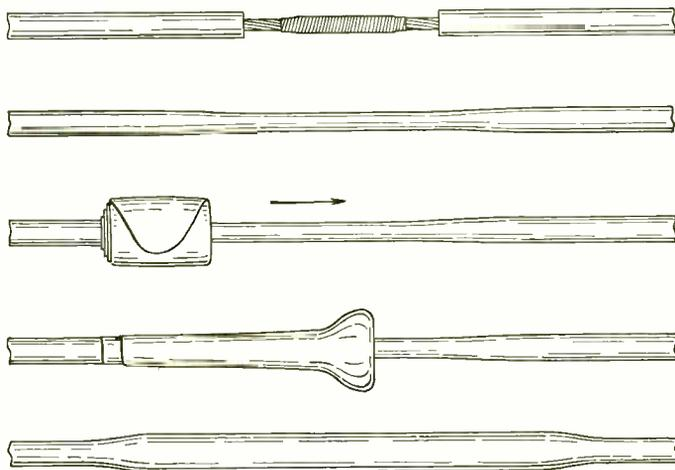
*Fig. 1—In splicing the gutta-percha insulation of a submarine cable by hand, the insulation at the two ends of the splice is drawn together, and a sheet of gutta-percha is wrapped around the cable and worked over the joint until it adheres at the seam and has a smooth outer surface*
