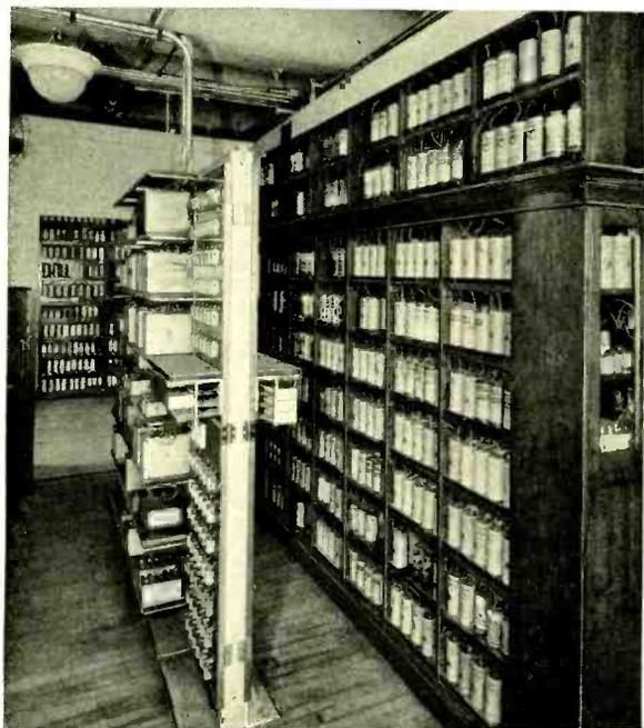
*Fig. 3—Part of the battery testing laboratory showing the methods of mounting the batteries on test*
