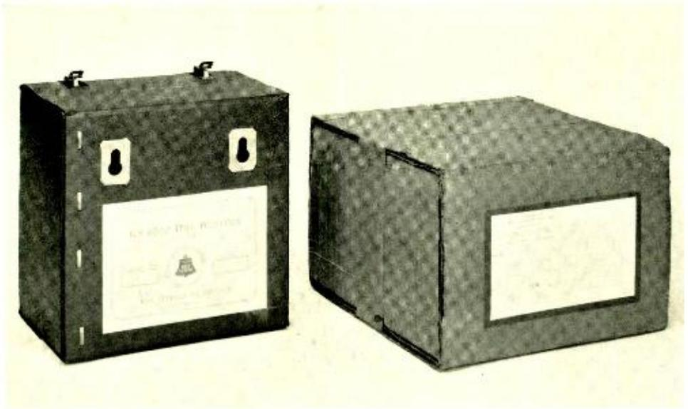
*To simplify the handling of dry cells for use at local-battery subscribers' stations, a new unit battery has been developed. A rugged black pulp board container shown above at the left, encloses three standard Blue Bell cells. The connections between cells of the battery are soldered and two spring terminals are provided so that connection may readily be made.*
