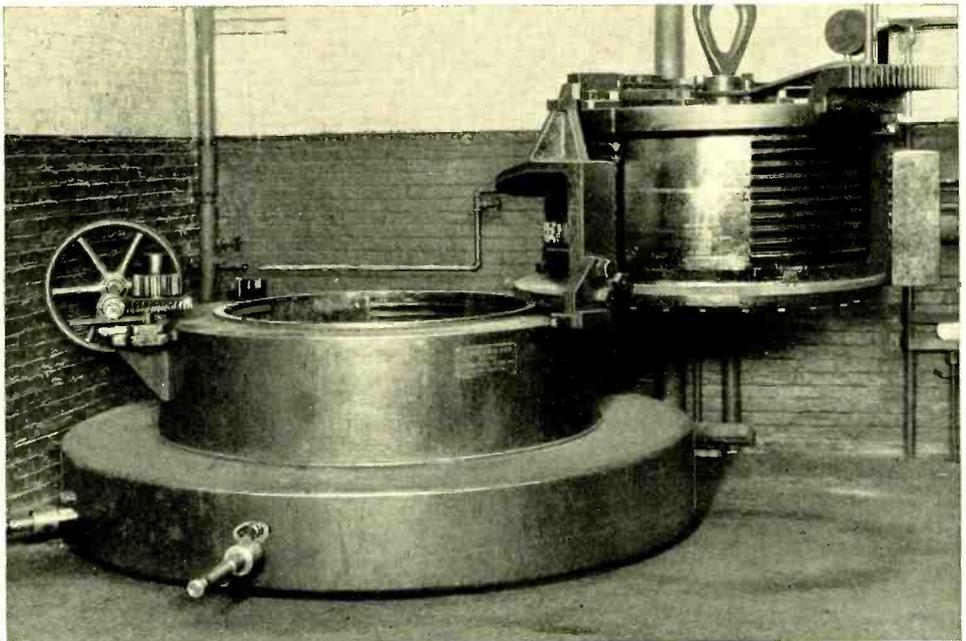
*Fig. 6—Equipment of this type was used at Norddeutsche Seekabelwerke for subjecting submarine cable cores to sea-bottom pressures and temperatures*
