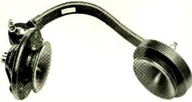
*Fig. 3—The first commercial handset was invented by R. G. Brown, and used by the Gold and Stock Telegraph Company of New York*
