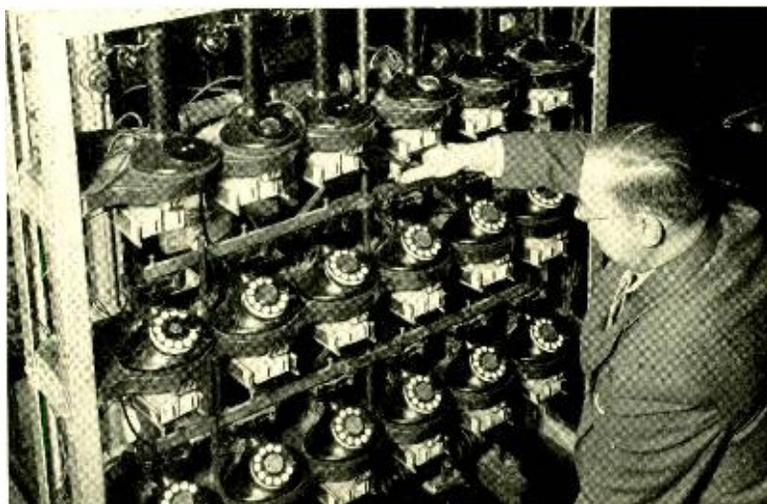
*This machine automatically tests the life of the switchhook contacts in eighteen telephone bases. It switches from one circuit condition for the break of the contacts to another for the make, and stops operating and lights a lamp when the resistance of any pair of contacts becomes objectionably high*
