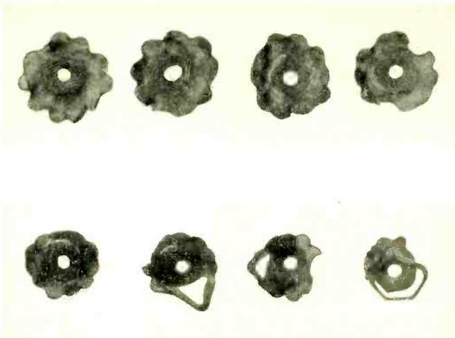
*Fig. 5—Machine made joints in paragutta insulation (above) cannot be pulled apart at the seam, as can some manually made joints (below)*
