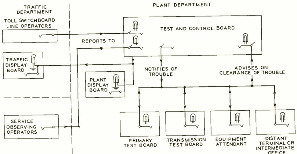
Fig. 1—How information regarding circuit conditions passes to and from the test and control board
