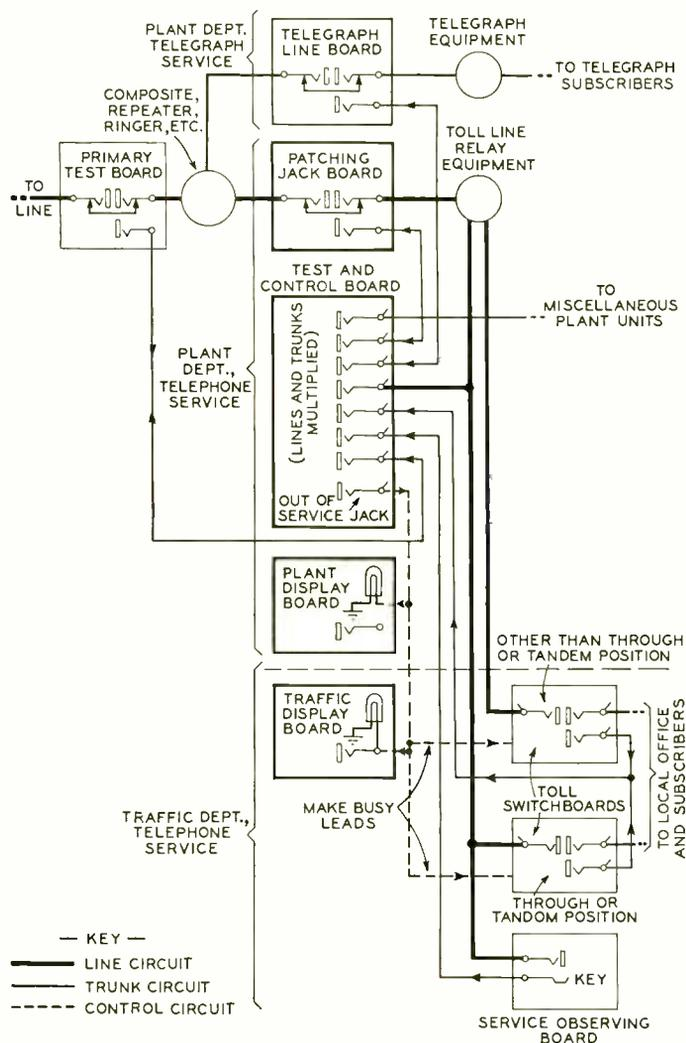
Fig. 2—How the test and control board is associated with other toll office units
