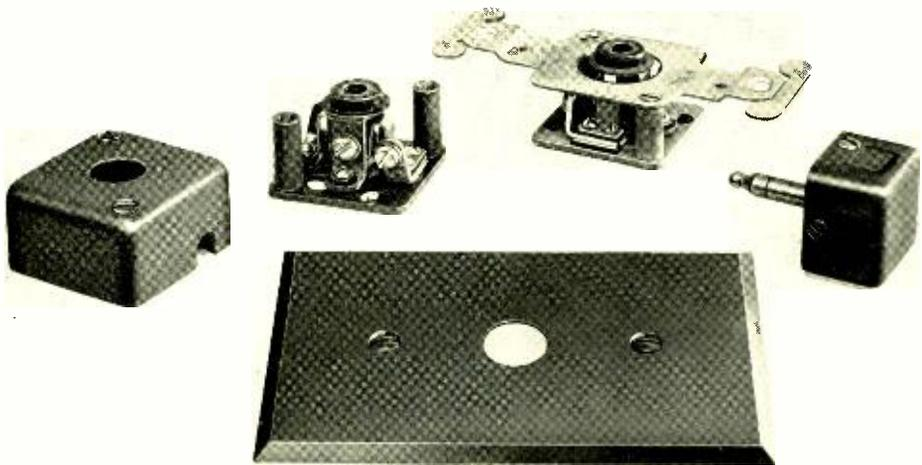
*Fig. 2—An ordinary switchboard jack is too long to be used conveniently for surface mounting, and so a shorter construction was provided. The body of the plug was shortened also*
