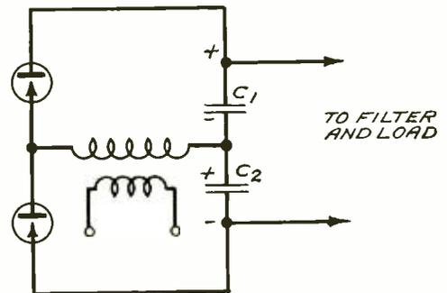
Fig. 5—A two-element rectifier for higher voltages
