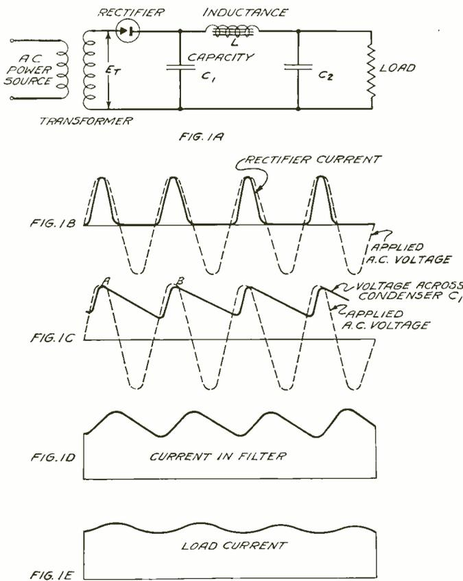
Fig. 1—A "half wave" rectifier; (a) its circuit; (b, c, d, e) wave-forms of current and voltage
