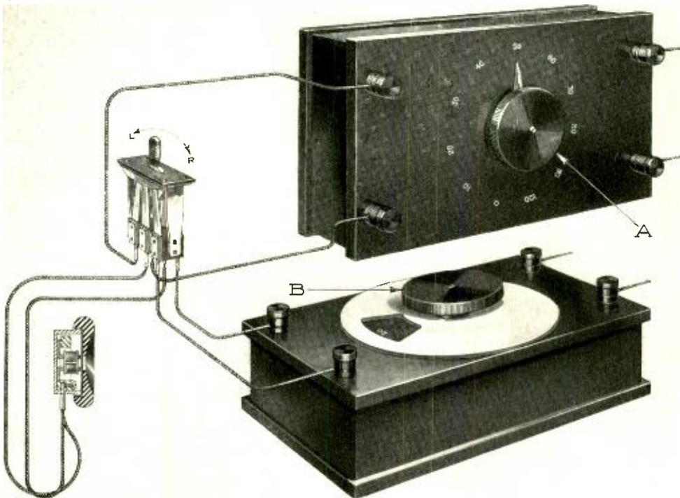
Fig. 1—The attenuators which vary the intensity of tone in the receiver. With the switch in left-hand position, "A" tone is heard; in right-hand, "B" tone is heard
