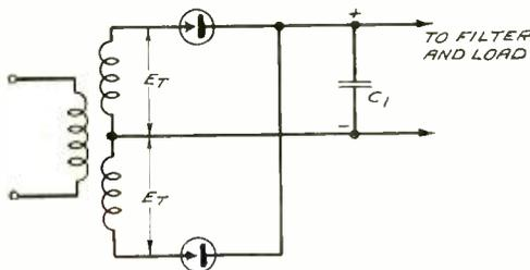
Fig. 3—A simple form of full-wave rectifier
