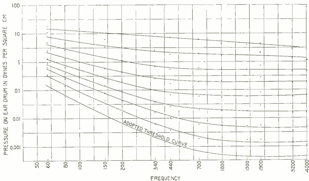
Fig. 2—Points on one of these curves represent, for the indicated frequencies, the physical stimuli which, acting on the ear drum, give sensations of equal loudness
