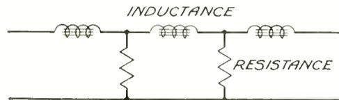
Fig. 7—Low-pass filter for filament circuits
