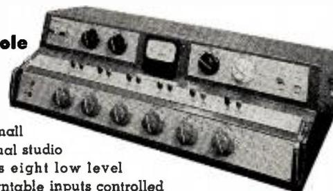
The 230B is the ideal console for small station or individual studio operation. It has eight low level microphone or turntable inputs controlled by four mixing controls and four line inputs controlled by two mixers. Its low height (9 3/4") provides maximum studio visibility. The controls are color coded and all parts are readily accessible. No other console in its price range offers as much as the Altec 230B.
