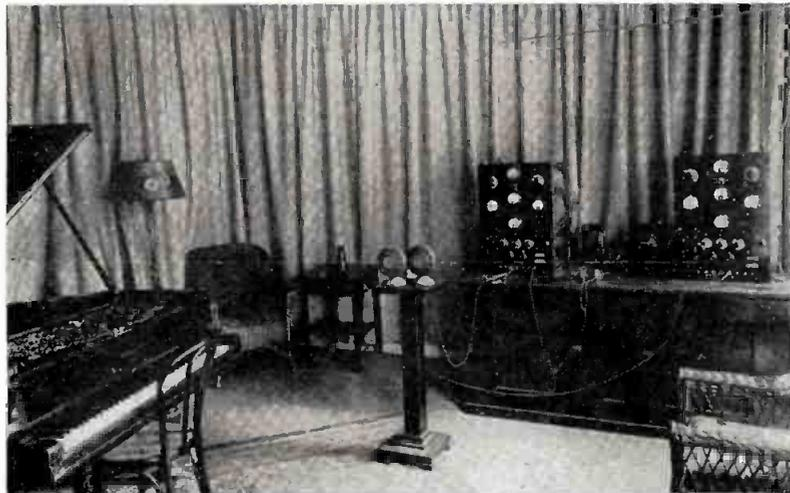
WDRG, operating as binaural station in 1924, shows studio containing right-ear and left-ear microphones and transmitters.
