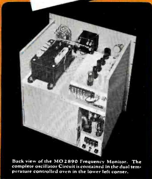
Back view of the MO2890 Frequency Monitor. The complete oscillator circuit is contained in the dual temperature controlled oven in the lower left corner.
