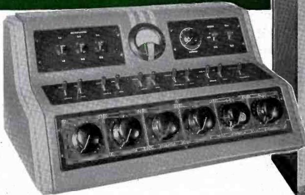
RCA 78-B1 operator's console control with switches for connecting preamplifier inputs to microphones in either of two studios, and mixer-outputs to either broadcast or auditioning channels. Other mixing circuits for turntables and remote lines. Illuminated V.I. meter may be set for either peak or RMS level or a VU meter is available if desired. 78-C1 is similar, but equipped for a single studio only, with 3 input channels but without audition keys.
