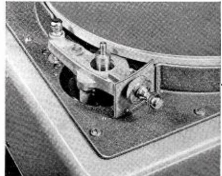
Unique Presto drive system. Step pulley on motor shaft drives against rubber tire on turntable rim. Lever changes speed instantly from 78 to 33⅓ RPM.
