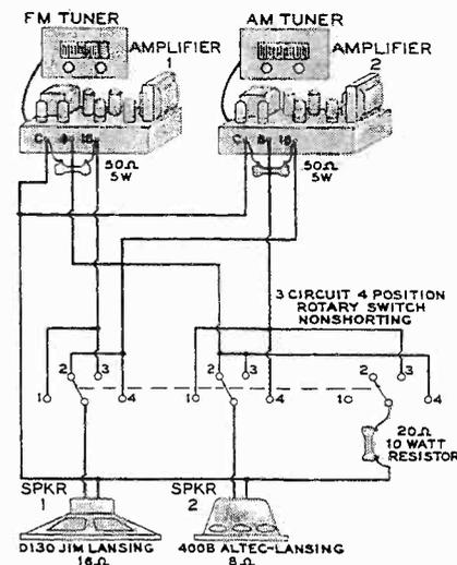
Speakers connect to either one or both amplifiers by this switching system.
