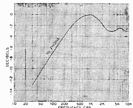
Fig. 2. Bass loss from ear response at 70 phons compared to 90-phon response. At low levels becomes thin and lifeless. A speaking voice reproduced louder than normal is enhanced with "broadcast boom." Bass overemphasis in male voices is well known; but it is scale distortion of the opposite variety, that which makes soft music sound empty, which most concerns the audiophile.
