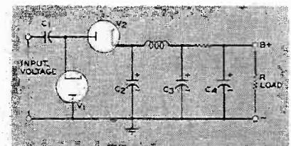
Fig. 4. A basic voltage-doubler circuit.
