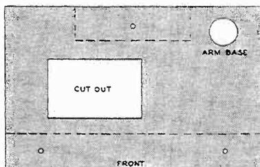
How the leveling screws are located on the turntable mounting board. Shelves beneath are indicated by dotted lines.
