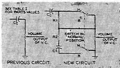
Fig. 5. Simple circuit boosts bass in background-music position of the switch.
