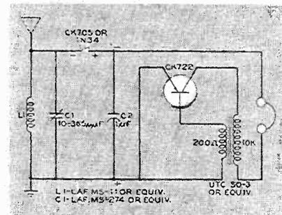
Fig. 2. A transistor audio oscillator operated by "free-energy" power supply.
