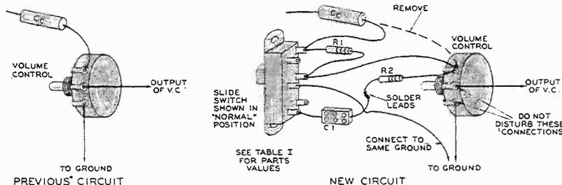
Fig. 6. How to interconnect component parts of the author's compensation circuit.
