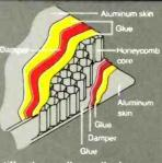
stiffer than ordinary diaphragms. This high rigidity makes it possi-ble to design a flat driver that is free of "cavity effect." The APM driver diaphragm is also well damped and exhibits virtually no internal resonances that can al-ter reproduction accuracy.
