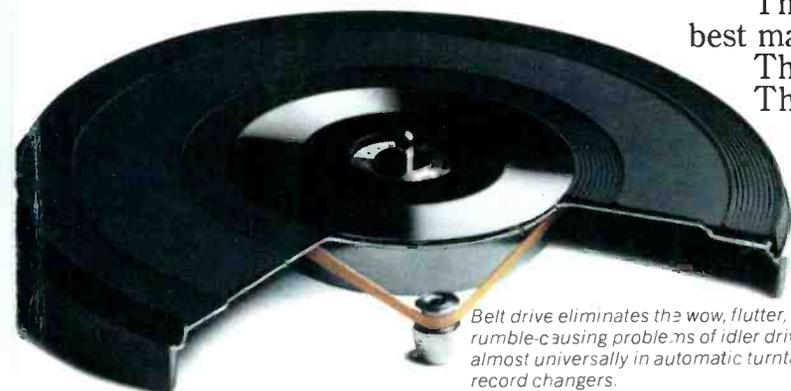
*Belt drive eliminates the wow, flutter, and rumble-causing problems of idler drives used almost universally in automatic turntables and record changers.*
