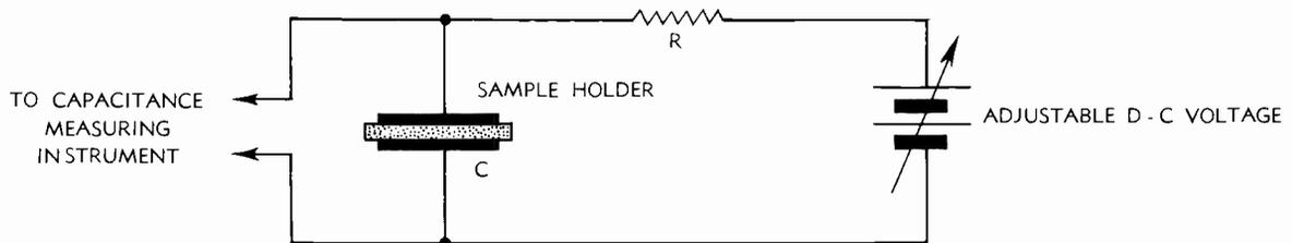
**FIGURE 4. ARRANGEMENT FOR APPLYING D C**
