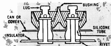
The molded cup employed on Aerovox motor-run capacitors prevents terminal
