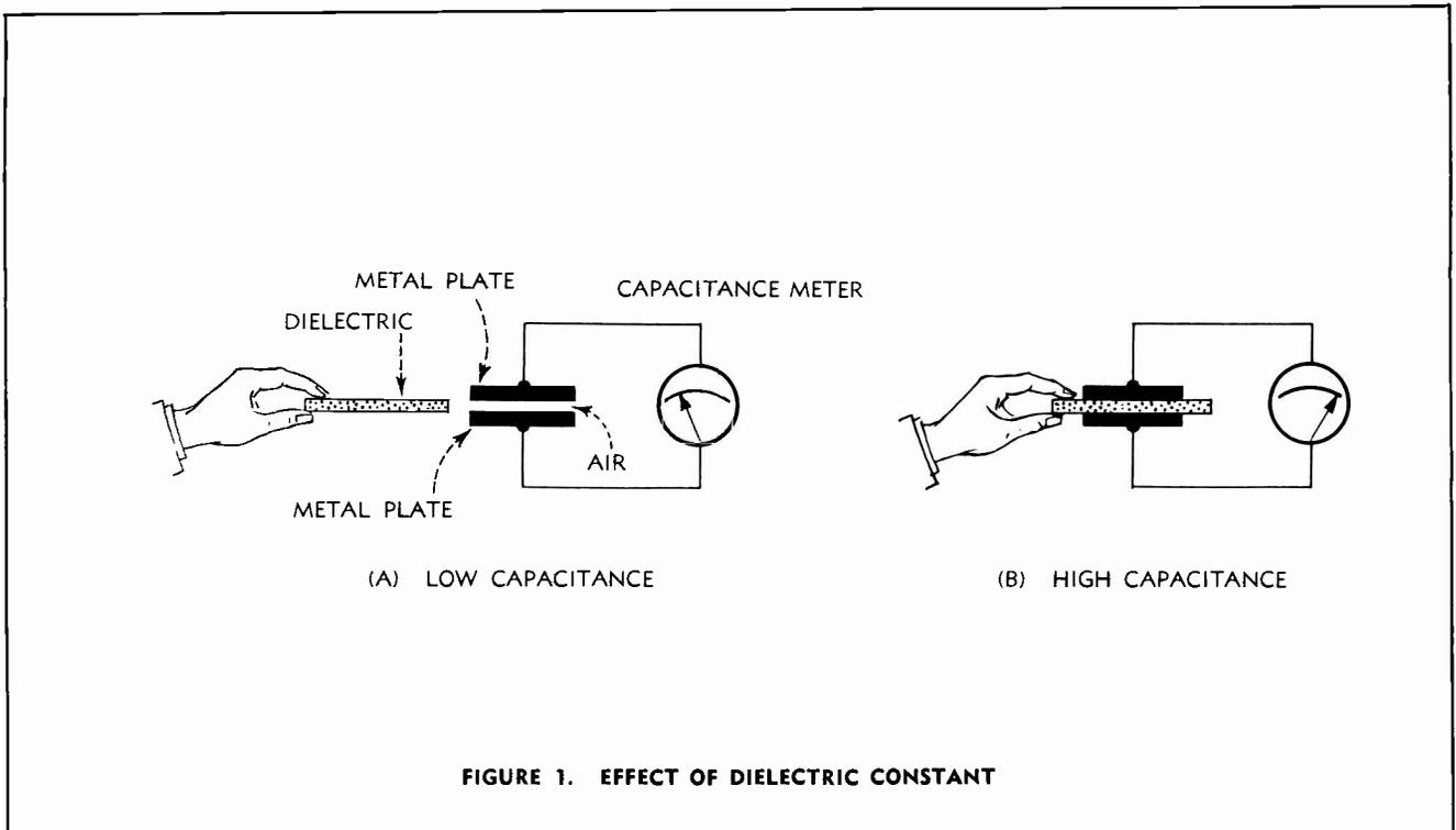
tive force is applied across the dielectric, and that a constant magnetomotive force acts upon the metal. Dielectric constant may also be expressed as the ratio of electrostatic flux density to field intensity.
