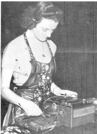
Final capacity test on paper capacitor.
