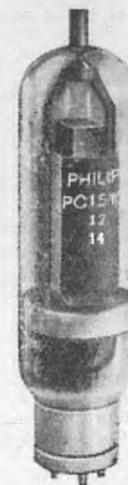
Penthode PC1.5/100 is the 100 watt model in the Philips Transmitting Penthode range, which already embraces 50 and 1000 watt models, and which will soon be augmented by a model with the hitherto undreamed-of output of 5 KW.
