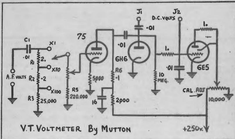
since most D.C. V.T. voltmeters are capable of measuring below .1 volt, which on the lowest range of our instrument is sufficient to close the shadow of the 6E5.
