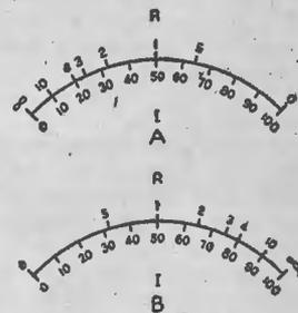
Fig. 3 - Typical ohmmeter scales applied to a milliammeter. The reversed scale at A occurs when the unknown resistance is connected in series, while the scale at B is of the type which results when the unknown resistance is connected in parallel with the meter.
