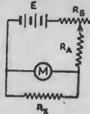
sistances. In this arrangement the unknown resistance is connected in parallel with the meter instead of in series, the meter resistance serving as the standard. Before the unknown resistance,  $R_X$ , is connected, the circuit current is adjusted to full-scale meter
