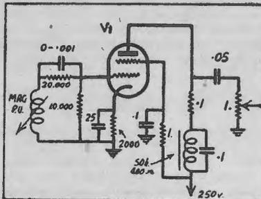
Another method of arranging bass correction by using a tuned choke in series with the plate load of the first amplifying valve.
