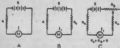
Fig. 1 - Basic ohmmeter circuits. The current first is measured with the known resistance,  $R$ , in the circuit of A. The unknown resistance,  $R_x$ , is then connected as shown at B and the new current noted. The unknown resistance may then be calculated by the formula given in the text. C shows the addition of a variable resistance,  $R_b$ , to compensate for battery deterioration.
