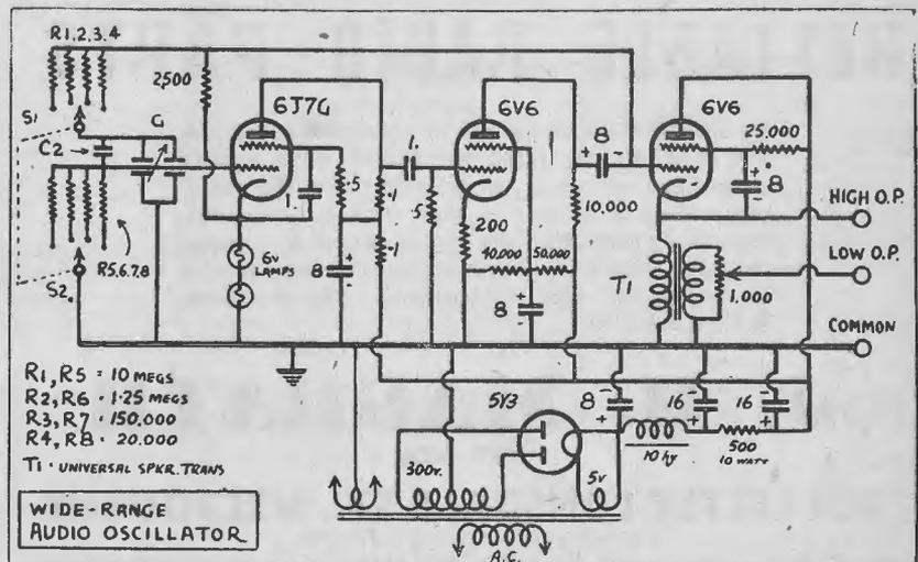
Circuit schematic for the handy audio oscillator.
