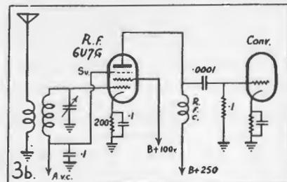
Diagram showing use of untuned r.f. stage.
