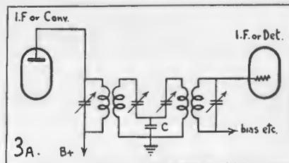
Circuit for Band-pass I.F. Channel.
