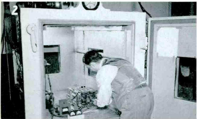
(2) Aircraft radio equipment built by RCA is put through rigid tests in the rarefied atmosphere of an altitude chamber.
