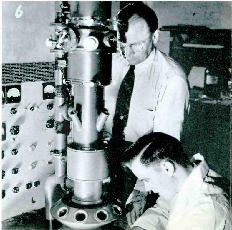
(6) The RCA Electron microscope, which can magnify up to 100,000 times, has opened the unseen, sub-microscopic world for exploration by the human eye.
