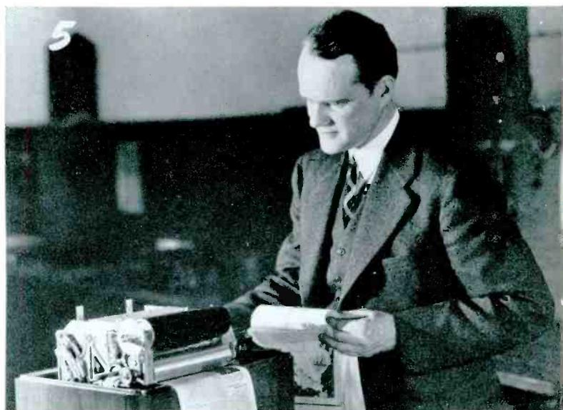
(5) Radio facsimile receiver-printer developed in RCA Laboratories for reproducing a newspaper by radio in home or office, or shipboard or in a plane.
