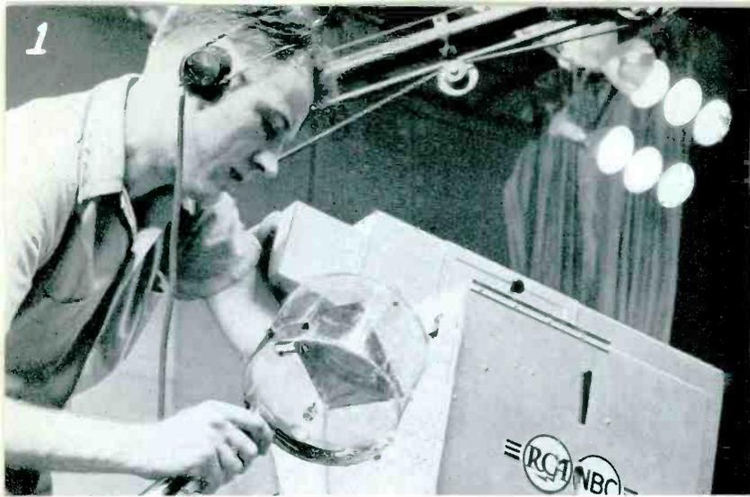
(1) The electronic eye of television, known as the iconoscope, is a development of RCA Laboratories.
