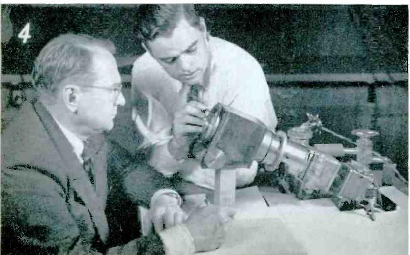
(4) Dr. V. K. Zworykin and Dr. James Hillier demonstrating an experimental model of new RCA portable electron microscope, 16-inches long and capable of magnification equal to that of the standard-size instrument.
