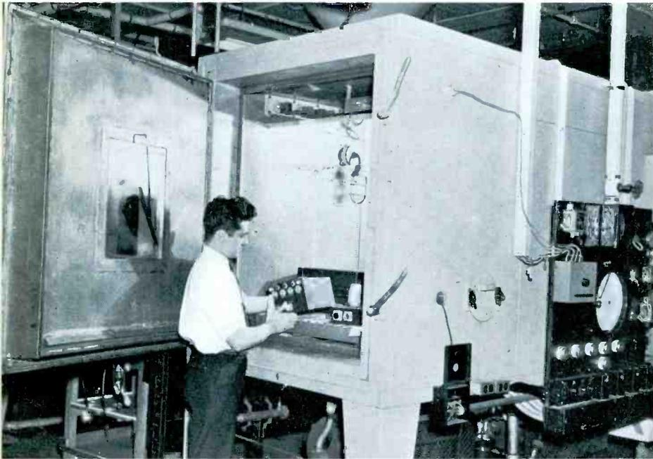
← To withstand the wide variety of climatic conditions to which radio sets are subjected in wartime, RCA receivers undergo tests of 152° heat and 22° below zero. In this chamber, humidity tests are applied.
