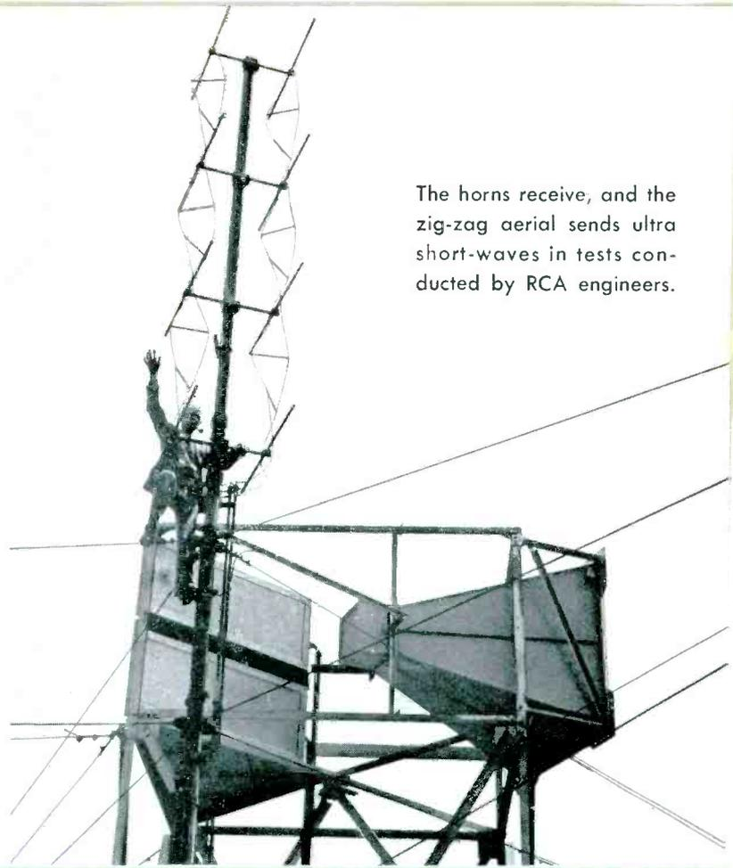
The horns receive, and the zig-zag aerial sends ultra short-waves in tests conducted by RCA engineers.
