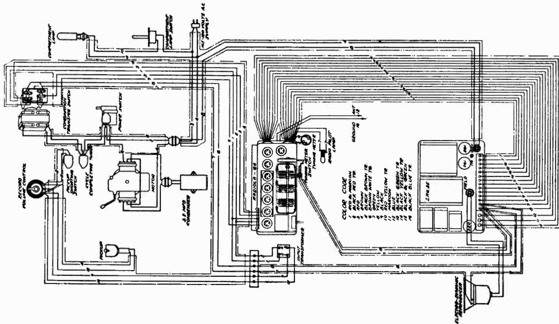
**Cable Wiring Diagram Automatic Electrola Radiola 9-54 above Serial No. 6441**
