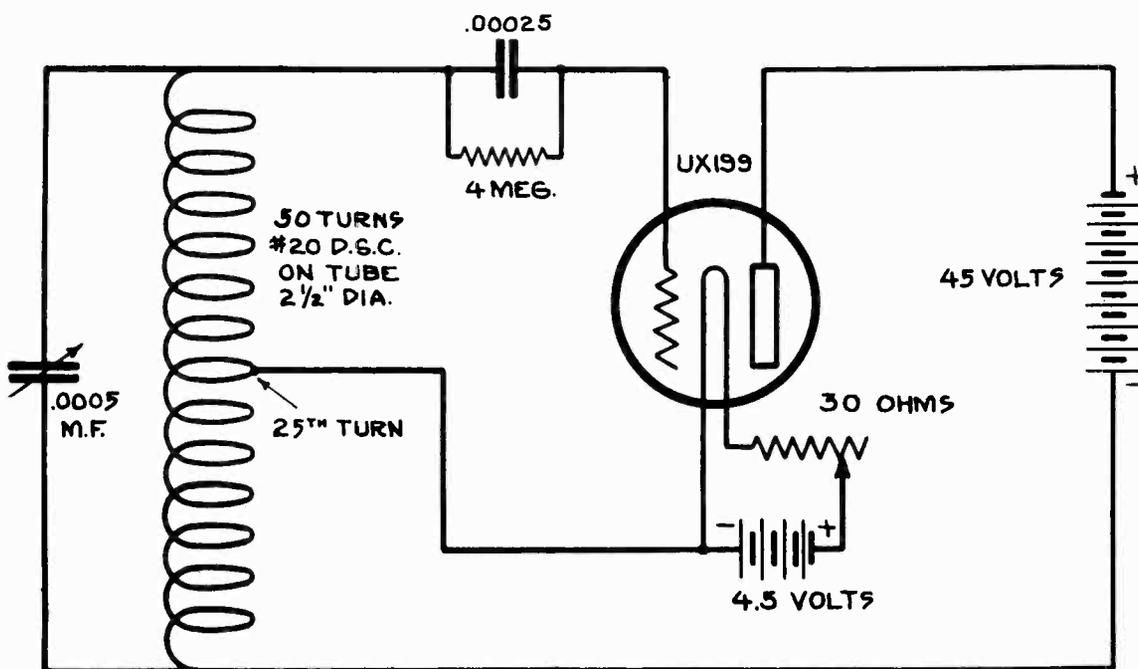
Figure 4—Wiring diagram of the modulated oscillator
