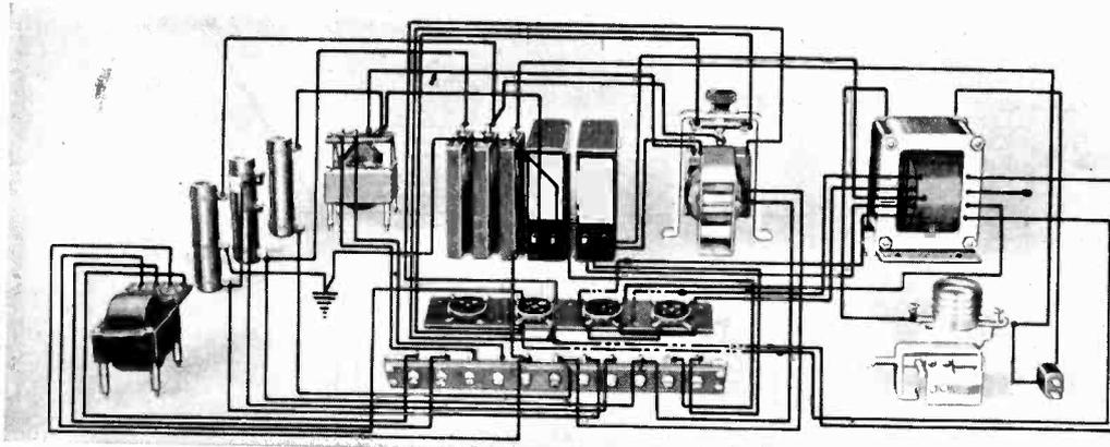
Parts and Wiring of Power-Amplifier Units
