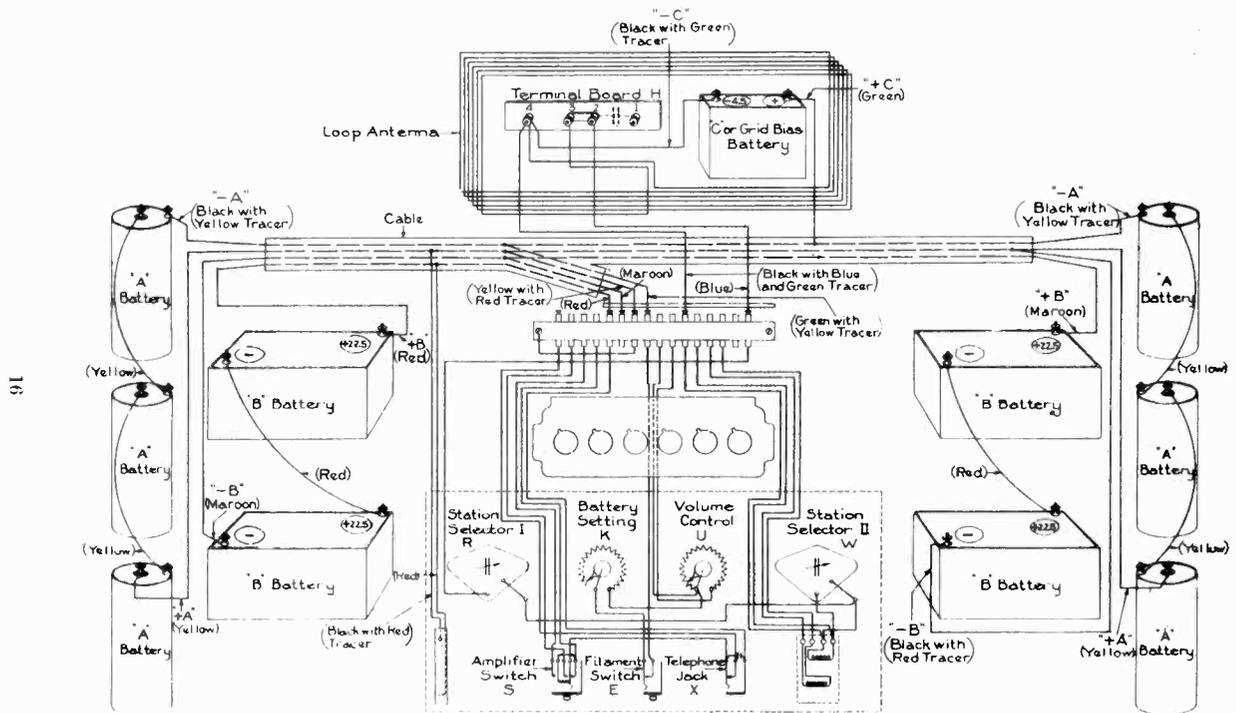
Fig. 6. Connection Diagram of Radiola Super-Heterodyne
