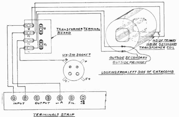
9-40 Input Transformer Wiring
