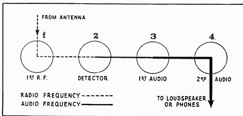
Figure 2—Radiotron sequence
