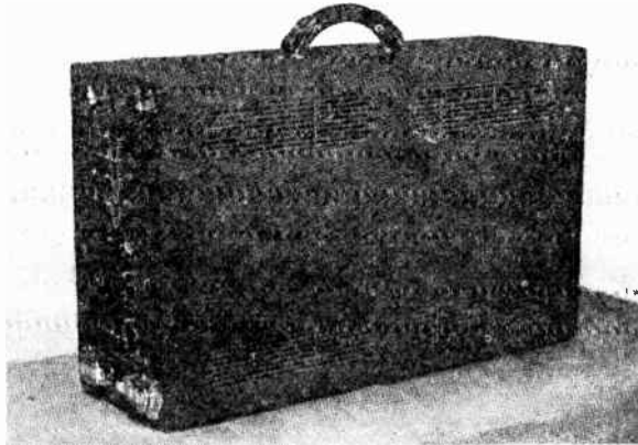
Fig. 4—Synchronizing-generator shaping unit with covers in place.
