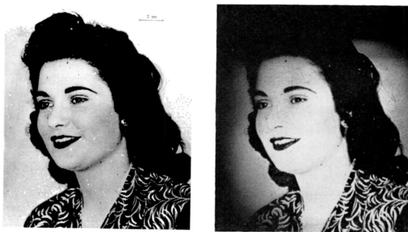
Fig. 12—Original and projected thermoplastic image. On the left is an enlargement from the photographic screened negative master and on the right is a rephotograph of the projected thermoplastic image ( 2 \times 3 feet) made from that master (see Reference (2), p. 207).
