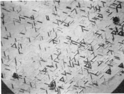
Fig. 2—Stacking faults in epitaxial layer on a silicon wafer not heat treated before deposition.
