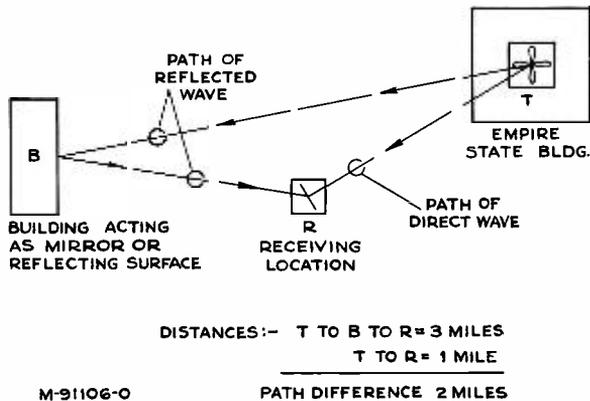
**Figure 22—Direct and Reflected Transmission Paths**
