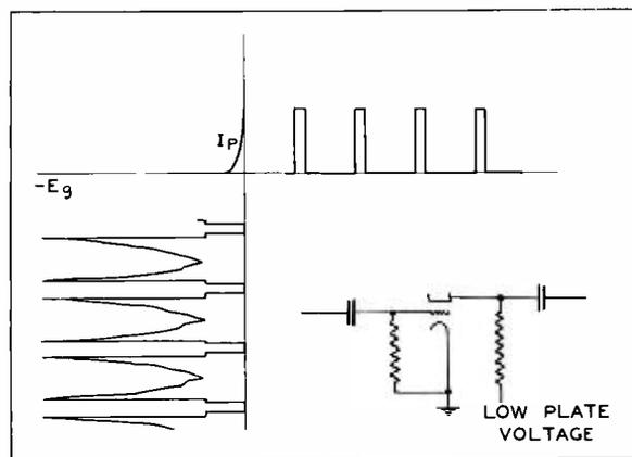
Figure 11—Operation of Synchronizing Separator
