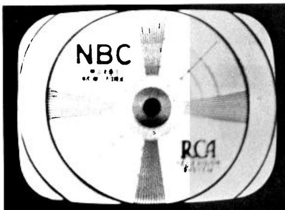
Figure 29—Focus Control Incorrectly Set
