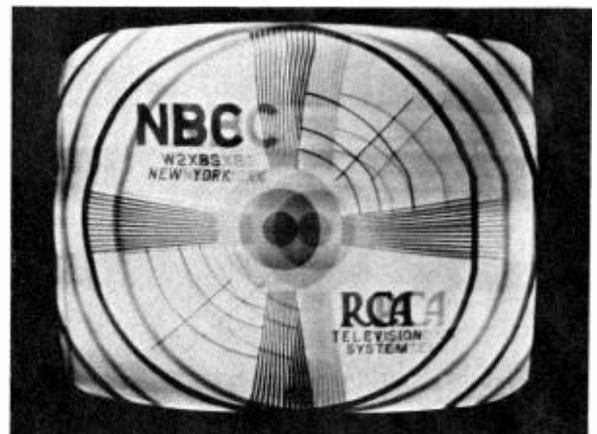
**Figure 24—Test Pattern Marred by a Reflected or Multi-path Signal**
