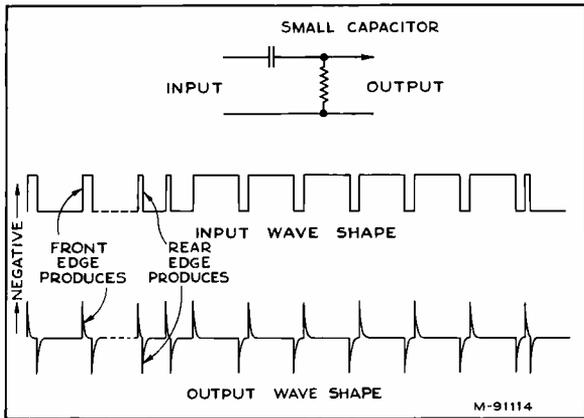
Figure 12—A Typical Horizontal Pulse Selecting Circuit and Wave-forms
