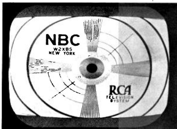
**Figure 37—Vertical Height Control Incorrectly Set**
