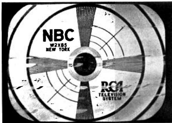
Figure 44—Excessive Auto Ignition Interference
