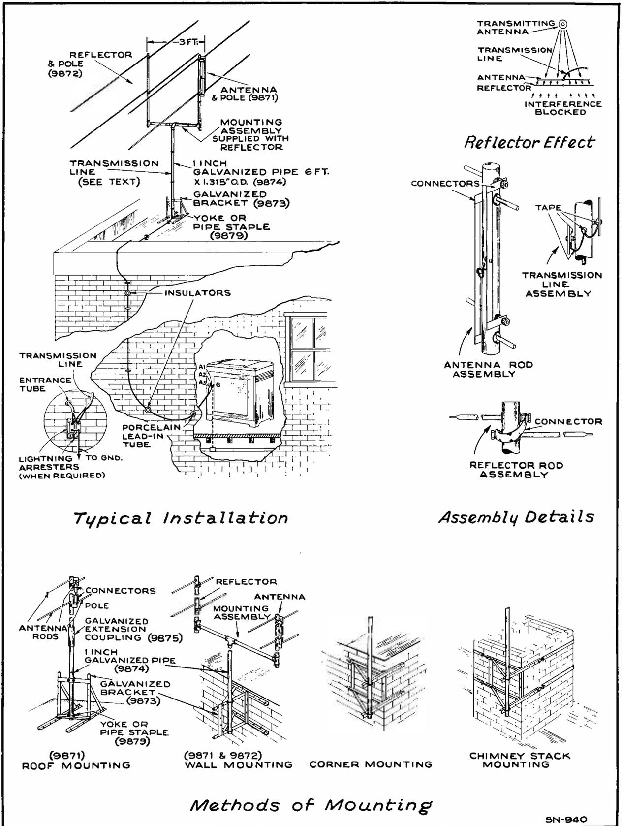
Figure 25—Typical Installation Details of RCA Double Dipole—Reflector Antennas
