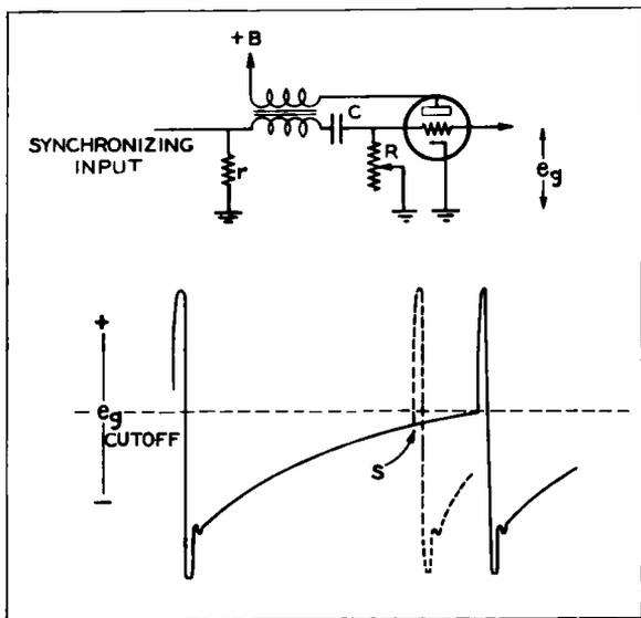
**Figure 15—Blocking Oscillator and Wave-form**
