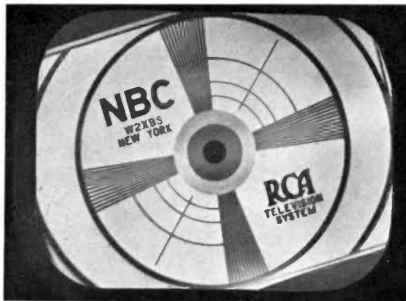
**Figure 34—Picture Incorrectly Oriented**
