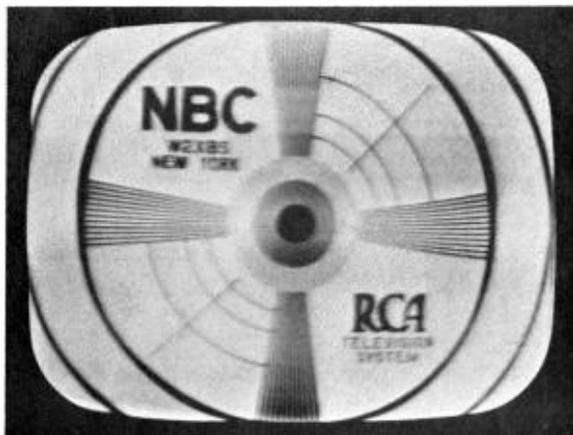
Figure 58—Loss of High Video Frequencies
