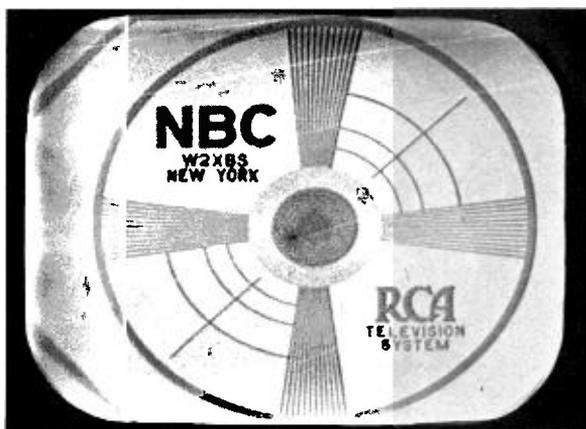
Figure 60—Effect of Damping Tube Failure
