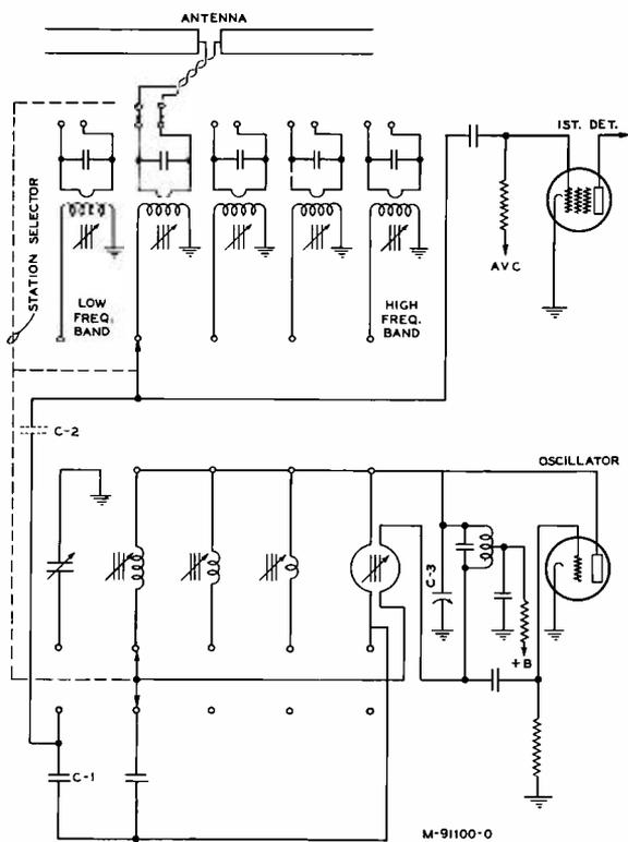
Figure 5—R.F. Input and Oscillator
