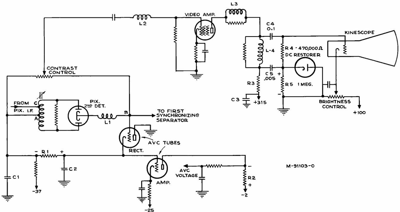
Figure 7—Picture Second Detector, Video Amplifier and D.C. Restorer
