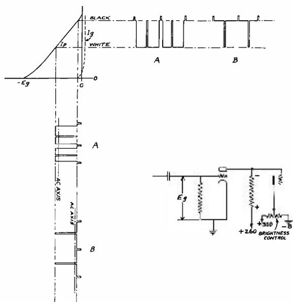
**Figure 9—Typical Grid Leak—
