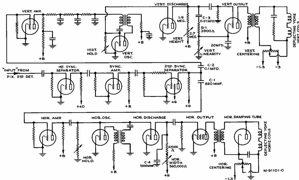
Figure 10—Synchronizing and Deflecting Circuits
