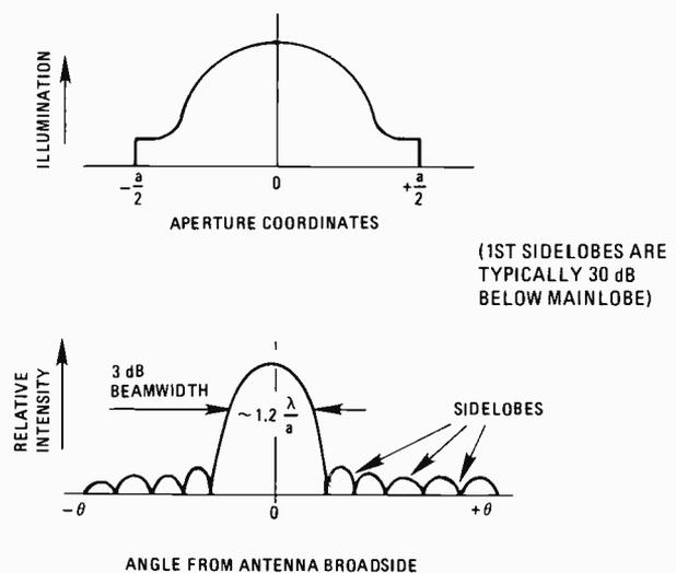
Fig. 17 Sidelobes are reduced by weighting the illumination across the antenna aperture. This weighting is accompanied by a slight broadening of the main lobe and a subsequent decrease in antenna gain.
