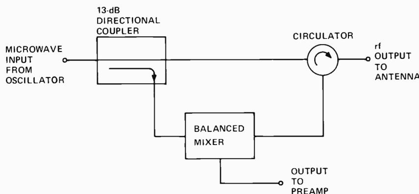
Fig. 5 **Microwave circuitry** sends and receives signals through same antenna, then produces frequency-difference output in mixer.
