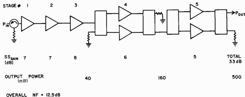
Fig. 3 Stage-by-stage performance of the GaAs FET amplifier. Pulsed operation takes place in the last two stages, where most of the power is dissipated.
