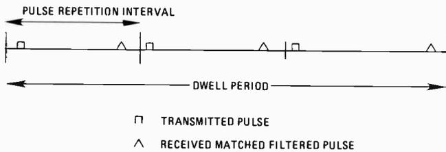
Fig. 9 Radar "dwell" enhances target detectability by processing a series of pulses.
