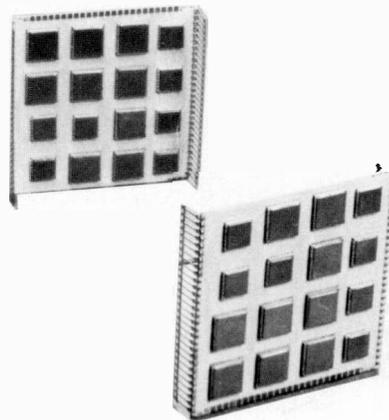
Mirror photograph of thick-film substrate interconnecting 16 chips on each side of the board. VLSI packaging densities will exceed 80,000 gates per square inch.
