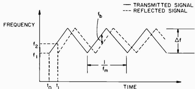
Fig. 4 Continuous-wave frequency-modulated system determines range by measuring the instantaneous difference in frequency between the transmitted and received signals. Because signal frequencies vary with time, frequency offset of reflected signal will depend on the time the reflected signal takes to return.
