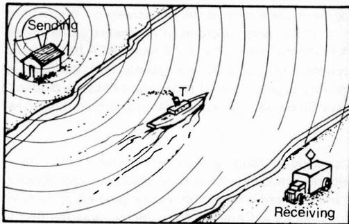
At the Naval Aircraft Radio Laboratory at Anacostia, D. C., Dr. A. Hoyt Taylor and Leo C. Young were conducting radio field strength measurements when they observed that a ship passing through a high-frequency field affected the performance of the receiver. In September 1922, they suggested the use of this interference effect for the detection of ships.
