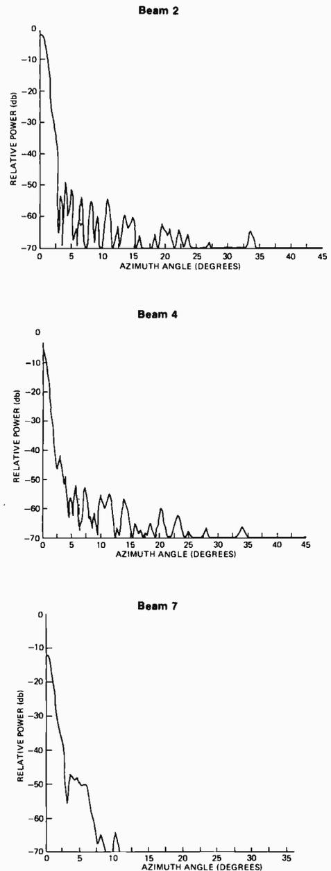
Fig. 5 Predicted azimuth patterns of elevation beam positions 2, 4, and 7 respectively. Achievement of low azimuth sidelobes is a primary objective of the antenna design. Computed patterns such as these, using the RCA simulation program DISH, guided the design to that end. Quantitatively, the objective is to provide azimuth sidelobe responses below -35 dB within 5° of the main beam, and below -50 dB outside of that azimuth angle region.
