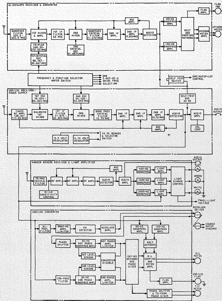
Fig. 3—AVN-210 VHF integrated navigation system.
