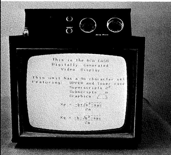
Fig. 3—Digitally-generated video (DGV) symbols as typically generated on a TV screen. White characters on a black background can also be produced.
