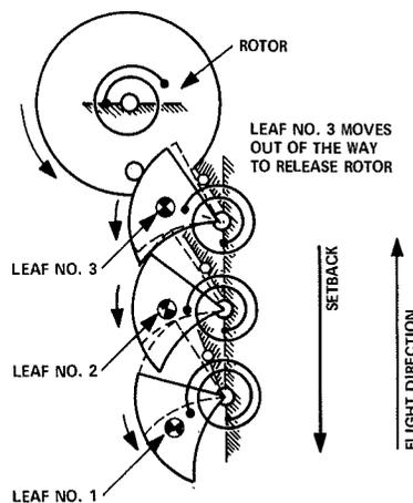
Fig. 2—First-order integrating accelerometer.
