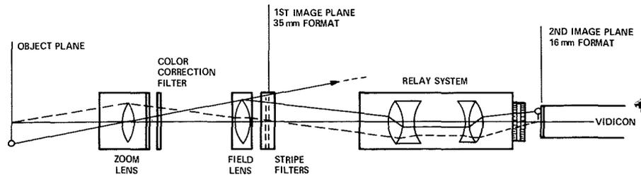
Fig. 6—Optics of 1-vidicon color camera system.
