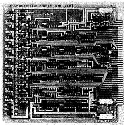
Fig. 3—Comparison of a closed-circuit TV generator using tubes (top left) with the solid-state monoscope circuitry used in the 6050 Video Terminal (top right). Bottom right is one of several integrated-circuit logic boards used in new data terminal for CSD to generate information for alpha-numeric displays.
