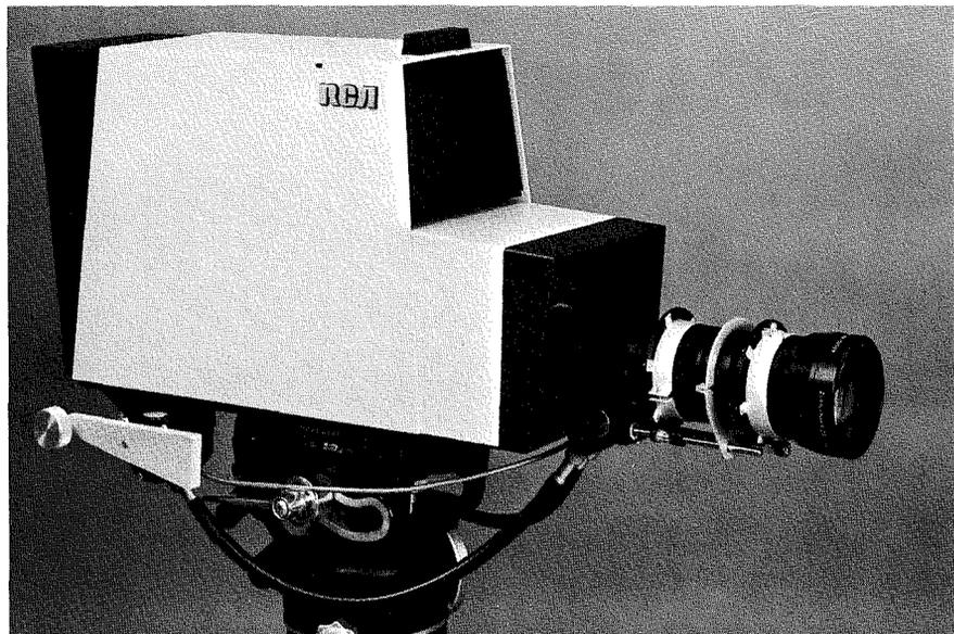
Fig. 1 (above)—One-tube color camera.
