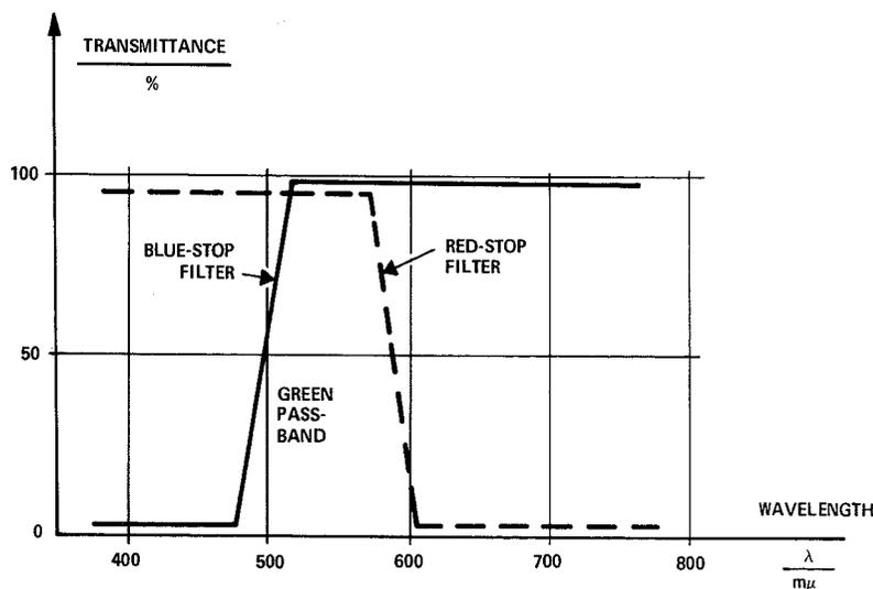
Fig. 4—Idealized dichroic-filter curves.
