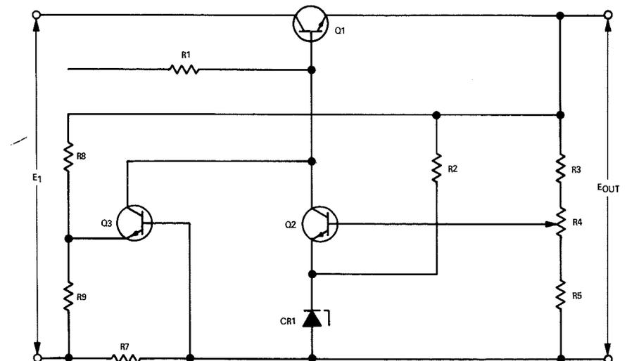
Fig. 5—A supply with foldback current limiting.
