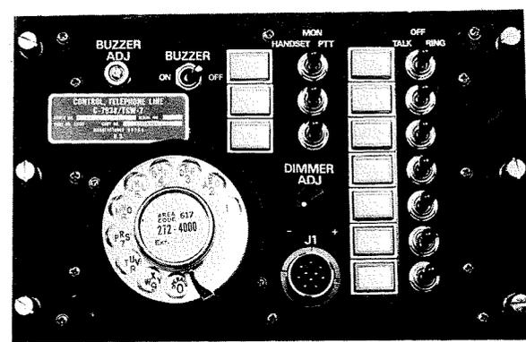
Fig. 4—Telephone control unit panel.
