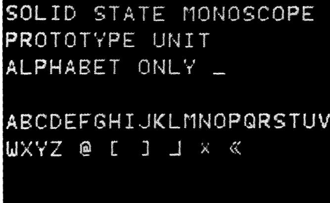
Fig. 4—Unretouched photograph of characters and symbols as generated by the prototype solid-state monoscope; the minor "glitches" are due to distortion in the vertical scan sine-wave and can be eliminated.
