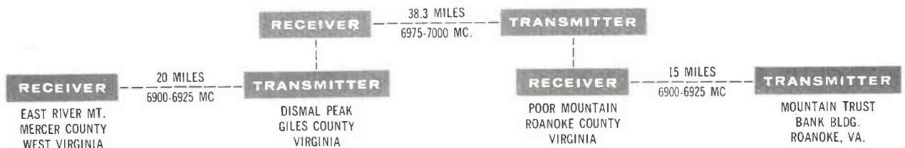
FIG. 5. Diagram of WHIS-TV Microwave system.
