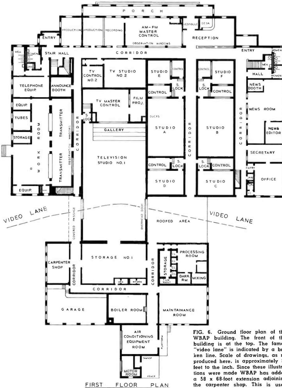
FIG. 6. Ground floor plan of the WBAP building. The front of the building is at the top. The famed "video lane" is indicated by a broken line. Scale of drawings, as reproduced here, is approximately 36 feet to the inch. Since these illustrations were made WBAP has added a 58 x 68-foot extension adjoining the carpenter shop. This is used as an additional storage space.
