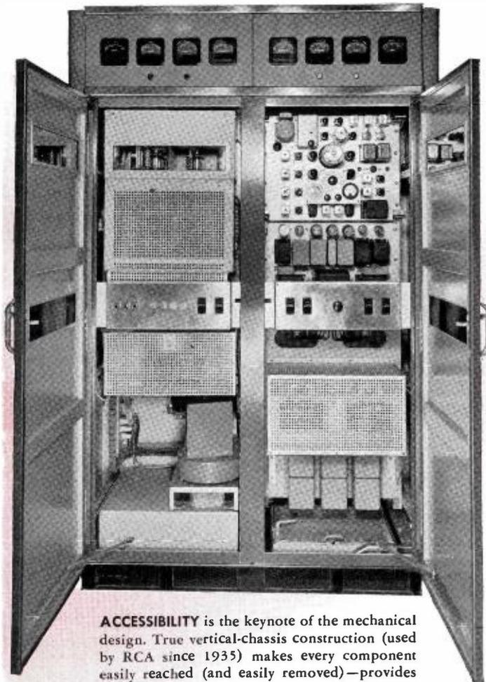
**ACCESSIBILITY** is the keynote of the mechanical design. True vertical-chassis construction (used by RCA since 1935) makes every component easily reached (and easily removed)—provides unimpeded up-draft ventilation. Unit-type assembly makes for easy installation, flexibility and simple modification for higher power.
