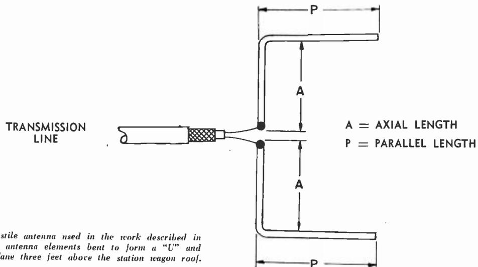
FIG. 1. The simplified turnstile antenna used in the work described in this article consists of two antenna elements bent to form a "U" and mounted in a horizontal plane three feet above the station wagon roof.
