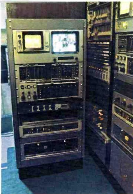
One of Opryland Productions' seven TK-45 cameras has a custom, rack-mounted CCU complete with test facilities, sync generator, and audio mixer. This rolling rack permits using the camera with the mobile unit or at the studio.
