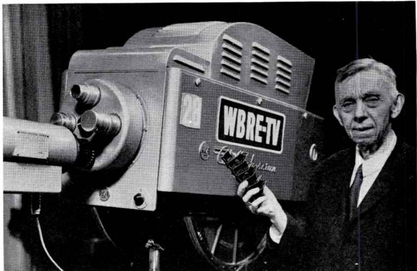
FIG. 1. Charles Sakoski, Sr., WBRE-TV Chief Engineer, holding one of the silicon rectifier stacks used in their new high voltage rectifiers.
