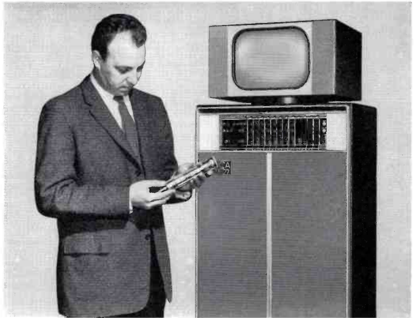
FIG. 17. Author, Dave Taylor, shows 1½-inch vidicon used for luminance channel in TK-27 Color Film Camera.
