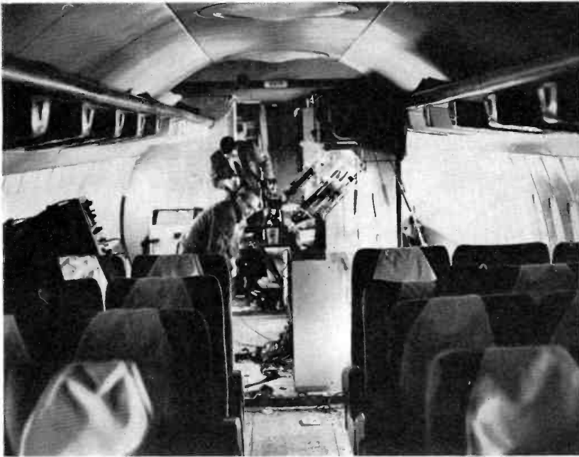
Seats were removed from the TWA Starstream to make room for the tape machines.
