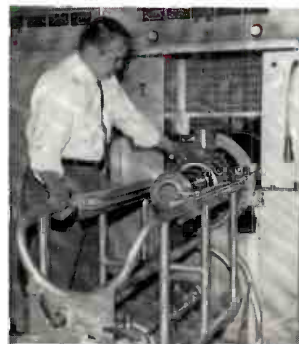
Klystron change is accomplished in only a few minutes with this unique carriage.
