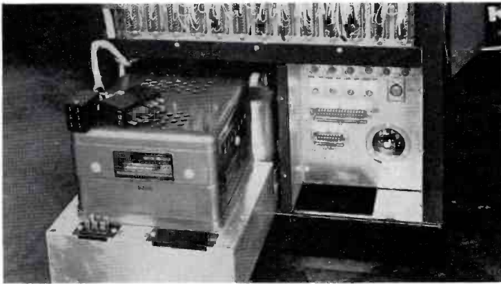
FIG. 9. Power deck of TR-3. At right is connector panel. At left is power supply.
