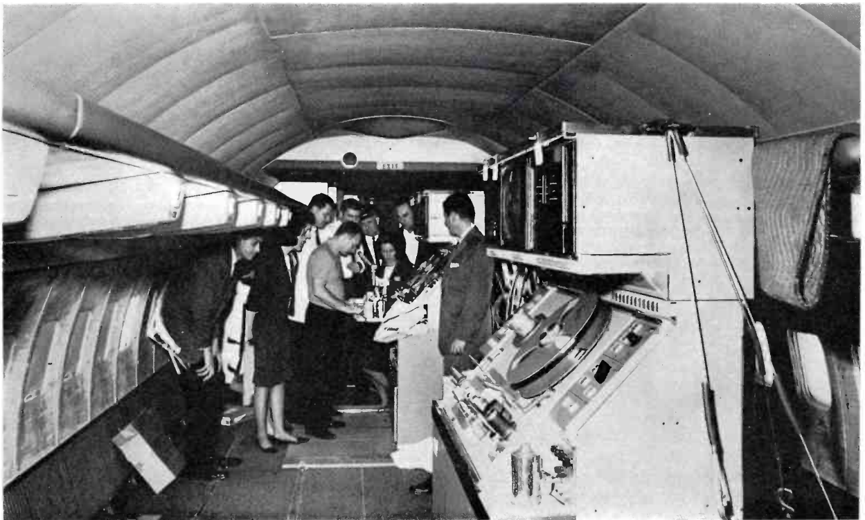
Seats were removed from the TWA Starstream to make room for the tape machines.
