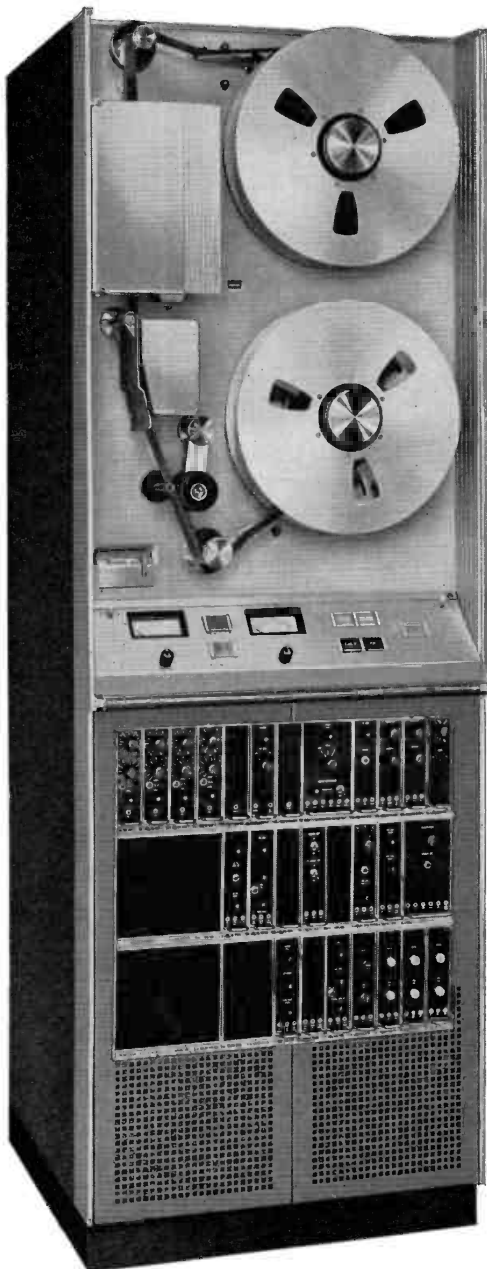
FIG. 6. TR-3 TV Tape Player, with bottom doors removed to reveal the modular construction.
