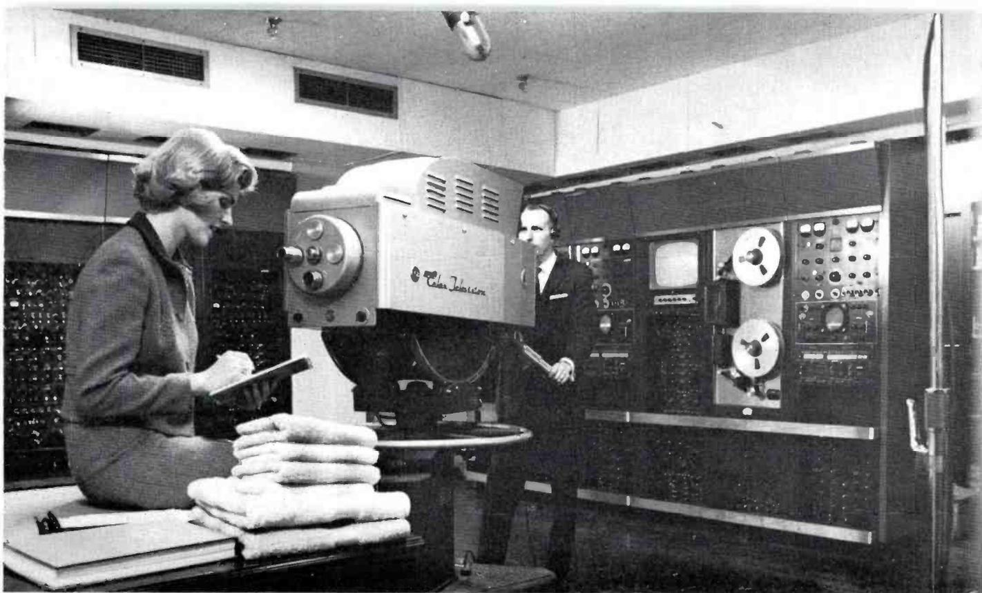
FIG. 29. Color recordings of simple commentary can be made by using the TK-41 live color camera.
