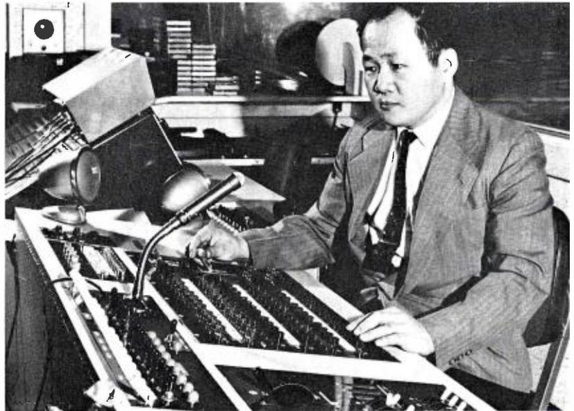
FIG. 2. Studio One control panel containing two special effects banks, two mixing banks, one preview bank and one line bank. Special effects selection panel is also incorporated.
