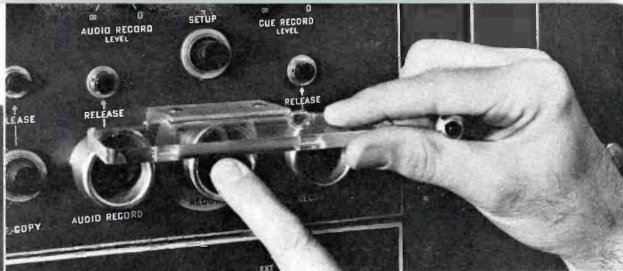
FIG. 15A. A special lucite cover built over the record buttons to prevent inadvertent operation of these controls and consequent accidental erasure.
