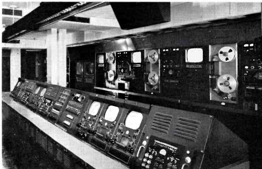
FIG. 10. Central control position of main console. Here all equipments can be put into the record mode, monitored and switched.
