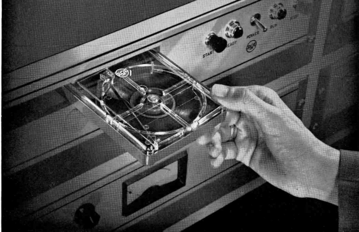
Here's the cartridge tape system with something new—*trip cue!* This unique feature allows you to record a special trip-cue tone that, during playback, can be used to start the next device in an automatic or semi-automatic system, with split-second timing. (In TV operations it may be used to advance slide projectors.)
