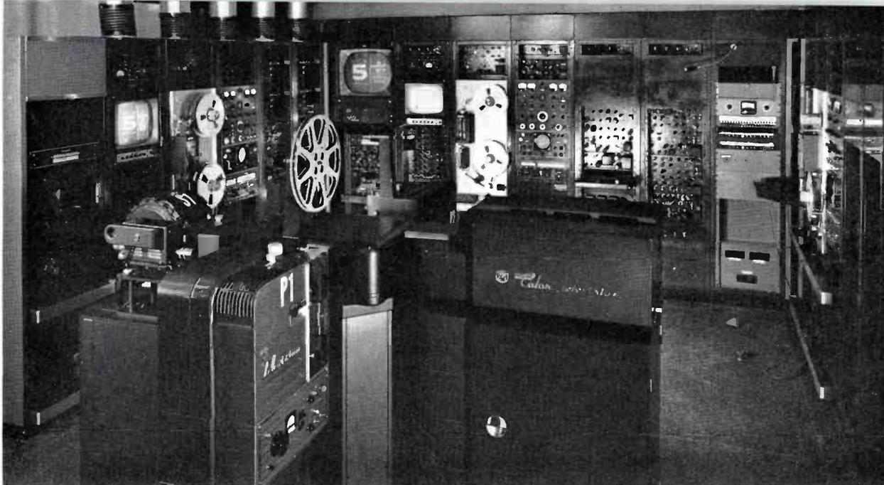
FIG. 21. In foreground is color TV film island. (There is also a monochrome film island.) Three TV Tape recorders are shown in U-shape background. All three are color recorders.
