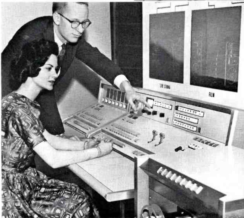
With the addition of other simplified controls, the basic switcher can also perform audio switching and provide special effects, as may be required. Operation can be completely automated with the addition of clock and memory units.
