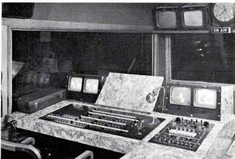
Our switcher is mounted in a console of my design. The console is constructed of wood and covered with a marble formica. An adjustable work-book rack and four eight-inch monitors are mounted directly to the back level of the console. A panel to the right of the TS-40 panel accommodates special effects selection, tv tape recorder, film projector, and slide projector remote control. We find this arrangement convenient, it also adds a stylish accent to our control room.
